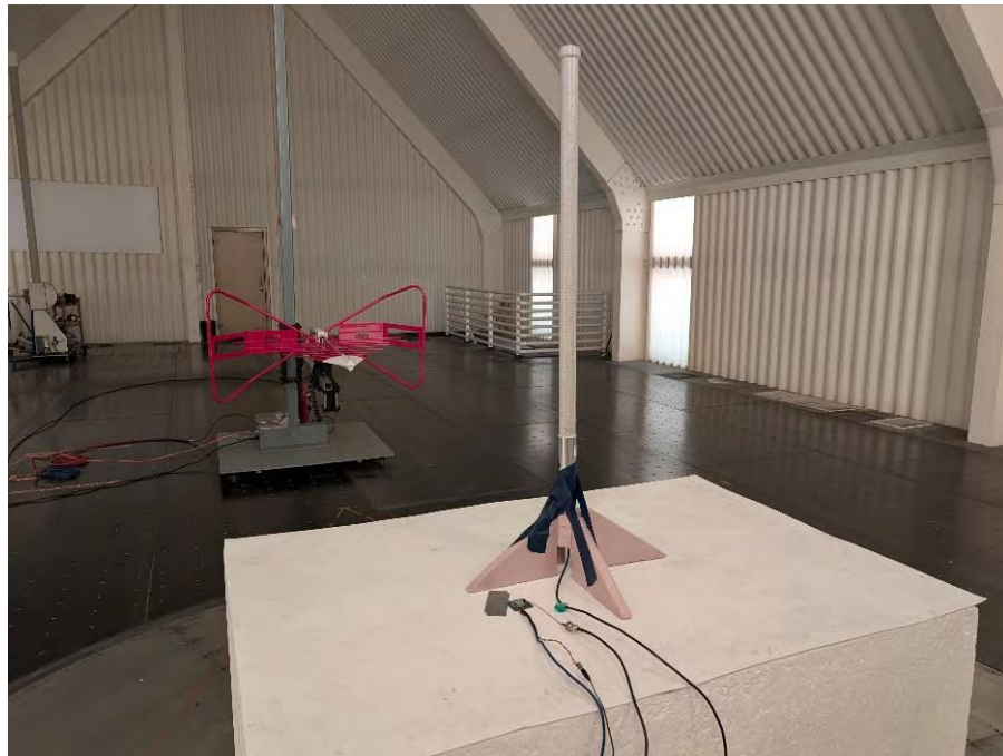
Photograph 18: Back View Radiated Emissions, Below 1000 MHz Worst Case Configuration with 2.4GHz Monopole Antenna
