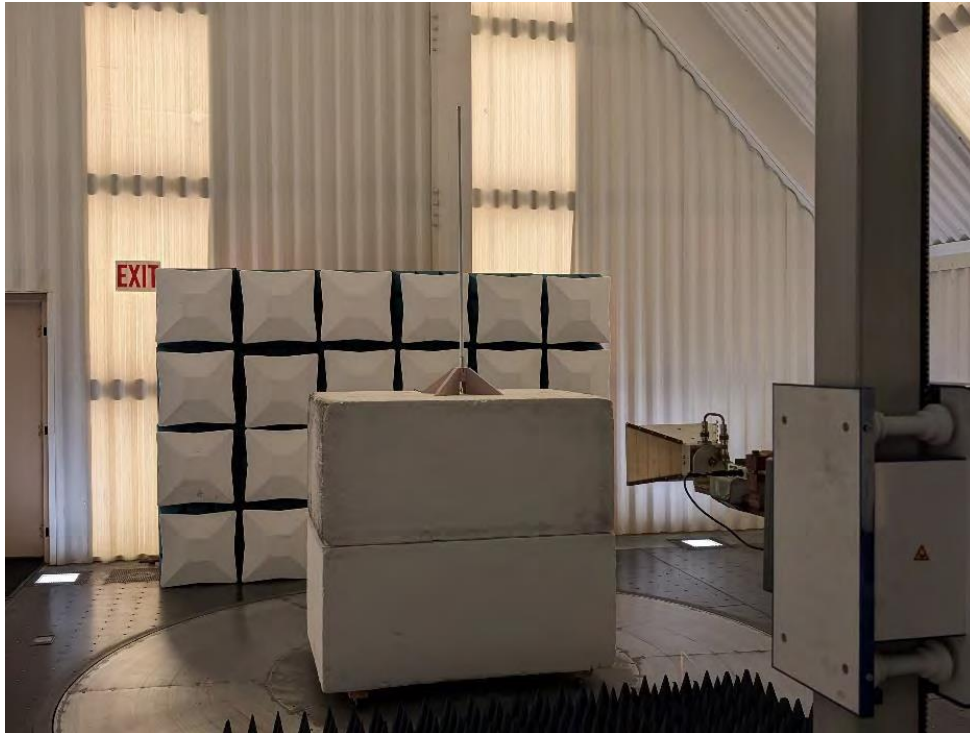
Photograph 7: Front View Radiated Emissions Worst Case – Above 1000 MHz Configuration with 900MHz Monopole Antenna
