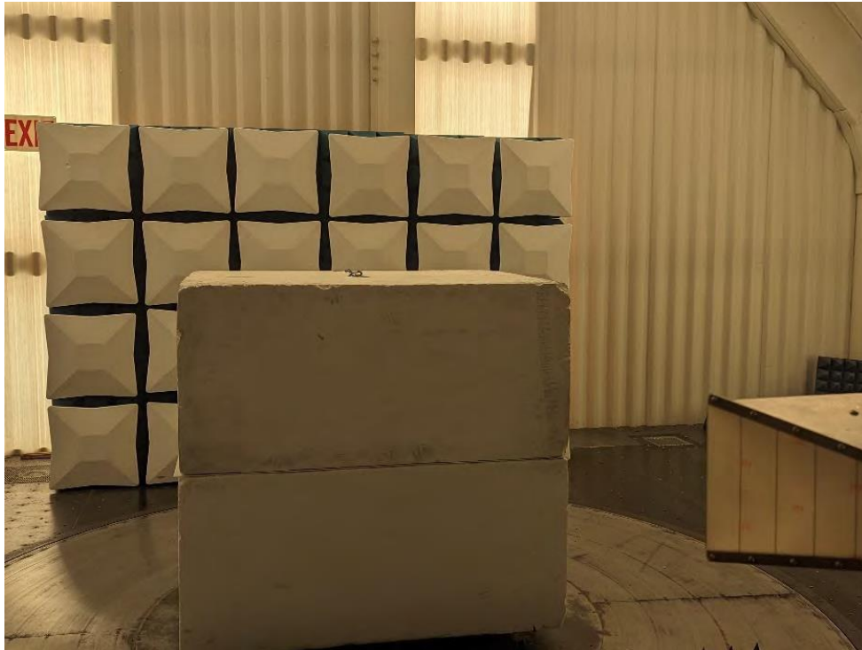
Photograph 15: Front View Radiated Emissions Worst Case – Above 1000 MHz Configuration with 2.4GHz Chip Antenna, Laying Flat
