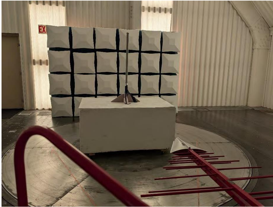
Photograph 17: Front View Radiated Emissions, Below 1000 MHz Worst Case Configuration with 2.4GHz Monopole Antenna
