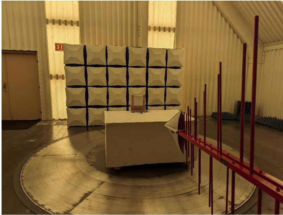
Photograph 9: Front View Radiated Emissions, Below 1000 MHz Worst Case Configuration with 900MHz Patch Antenna
