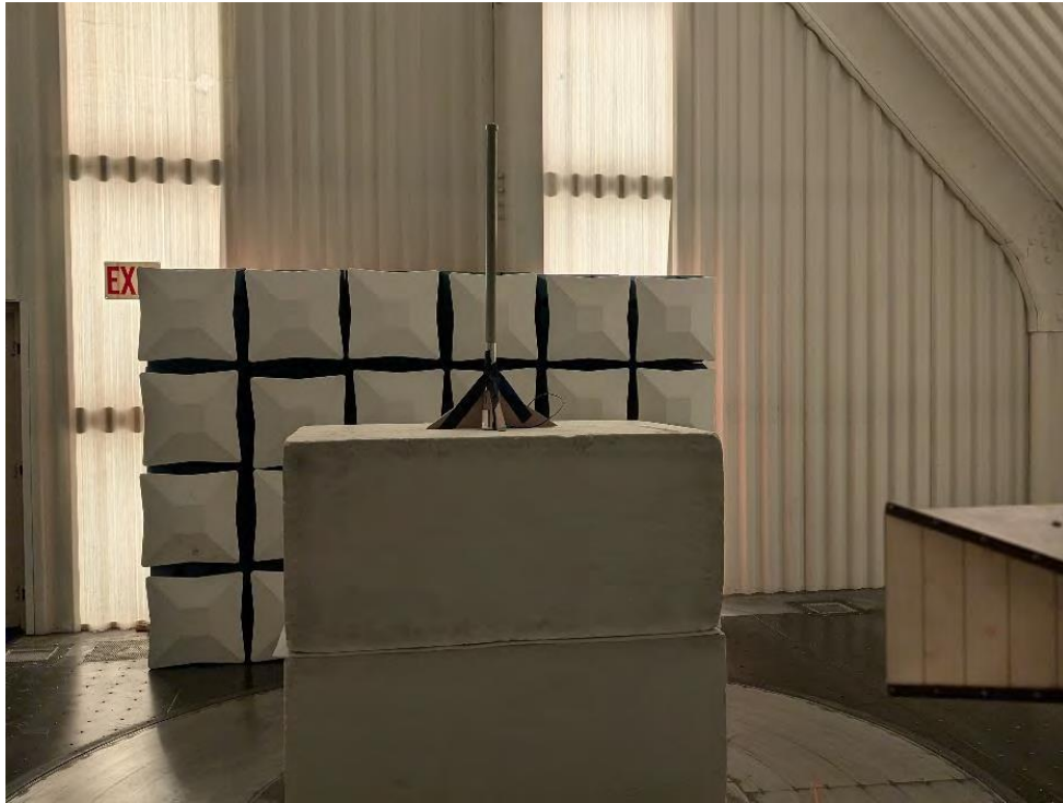
Photograph 19: Front View Radiated Emissions Worst Case – Above 1000 MHz Configuration with 2.4GHz Monopole Antenna
