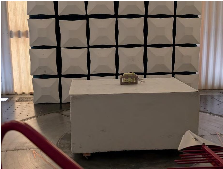
Photograph 1: Front View Radiated Emissions, Below 1000 MHz Worst Case Configuration with 900MHz Coil Antenna
