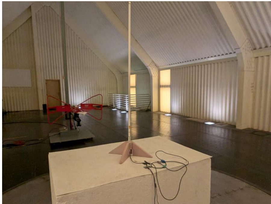
Photograph 6: Back View Radiated Emissions, Below 1000 MHz Worst Case Configuration with 900MHz Monopole Antenna
