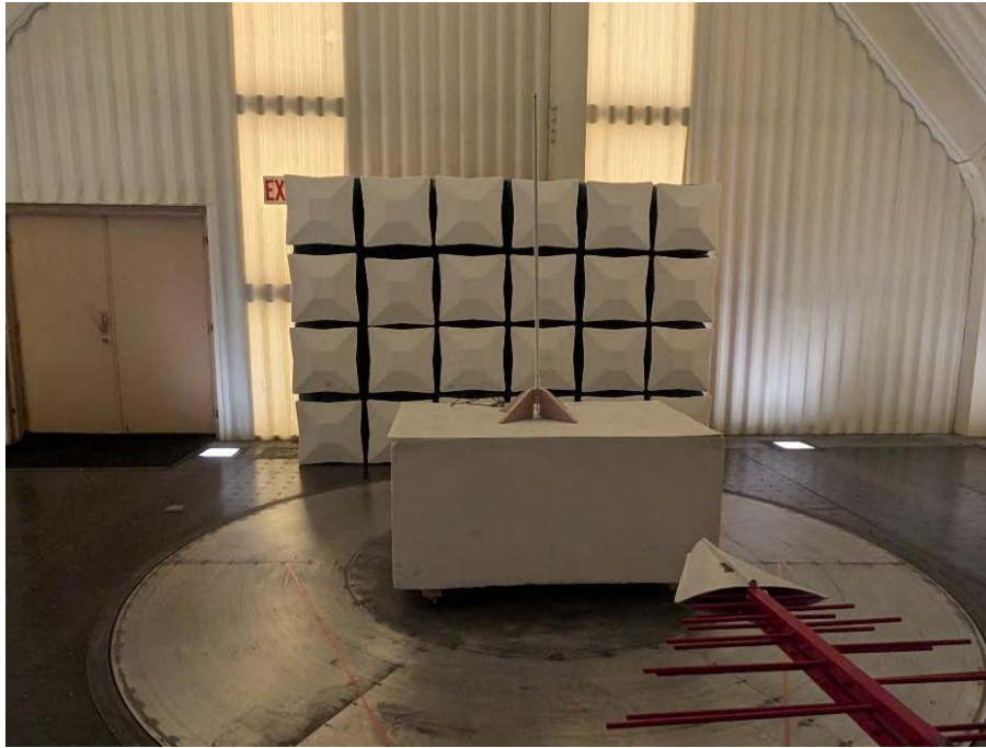
Photograph 5: Front View Radiated Emissions, Below 1000 MHz Worst Case Configuration with 900MHz Monopole Antenna
