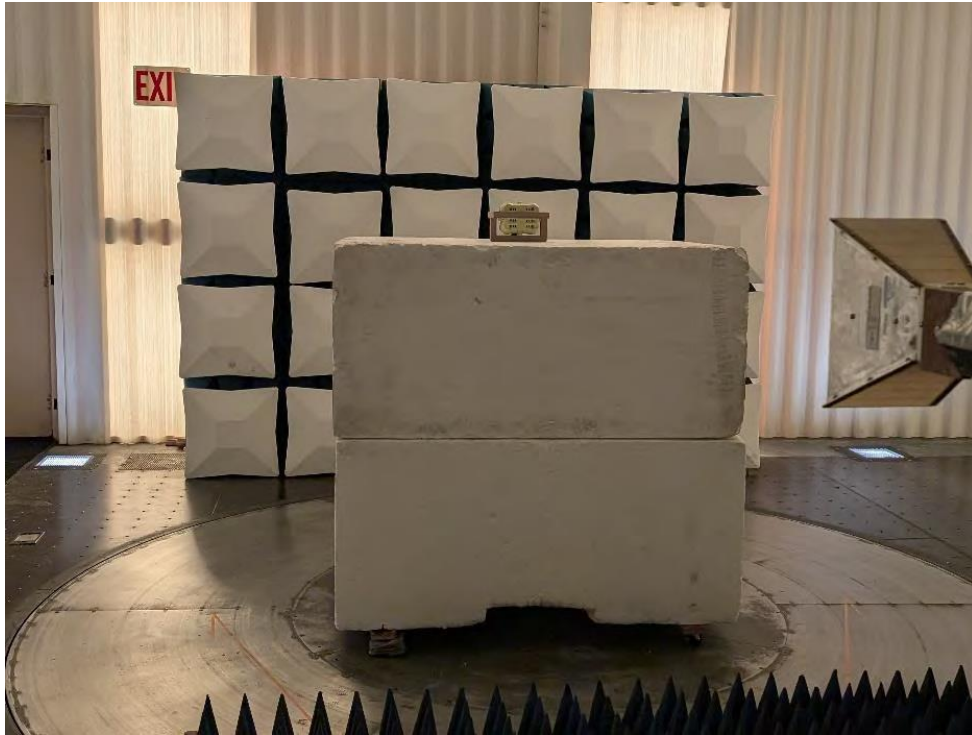
Photograph 3: Front View Radiated Emissions Worst Case – Above 1000 MHz Configuration with 900MHz Coil Antenna
