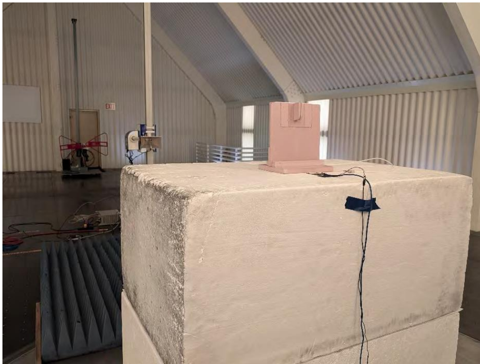
Photograph 12: Back View Radiated Emissions Worst Case – Above 1000 MHz Configuration with 900MHz Patch Antenna
