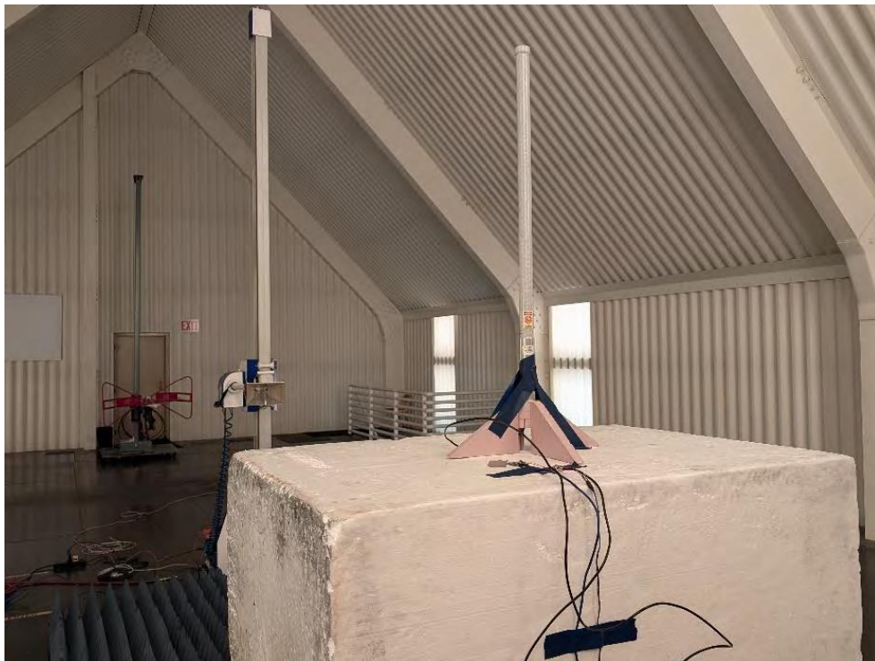
Photograph 20: Back View Radiated Emissions Worst Case – Above 1000 MHz Configuration with 2.4GHz Monopole Antenna
