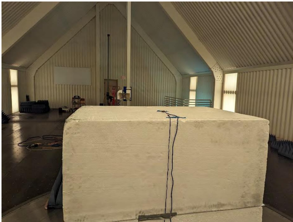
Photograph 16: Back View Radiated Emissions Worst Case – Above 1000 MHz Configuration with 2.4GHz Chip Antenna, Laying Flat
