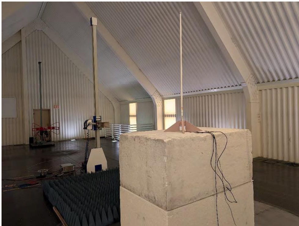
Photograph 8: Back View Radiated Emissions Worst Case – Above 1000 MHz Configuration with 900MHz Monopole Antenna
