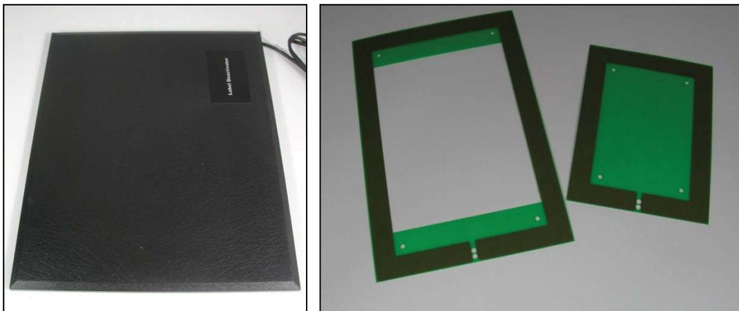
Table top deactivation pad on the left and two versions of an under-mount pad on the right.
