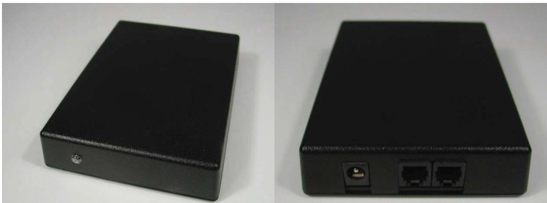
The Dual Deactivator Electronics is housed in an easy to mount casing. At the front there is an LED indicating power. In the rear there is the power connection and two connections for deactivation pads.
