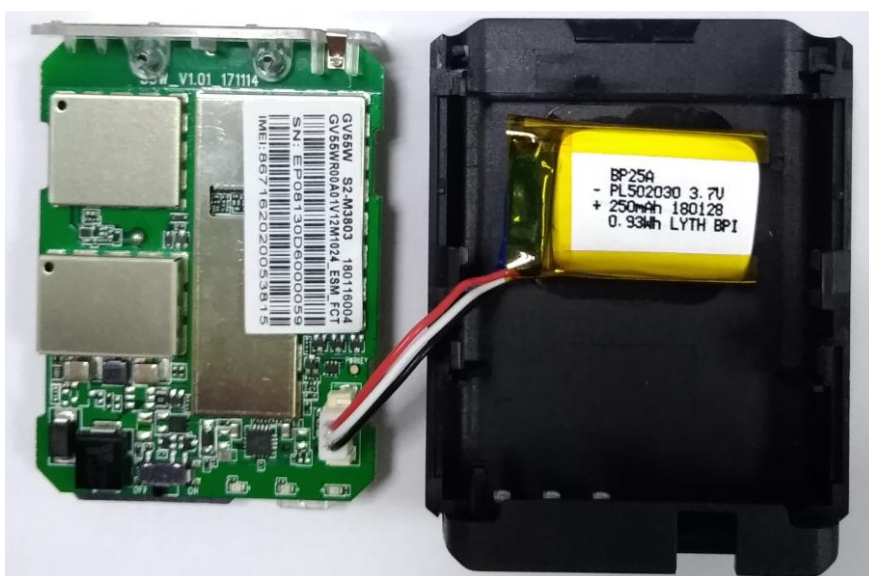
Figure 6. Backup Battery Installation
