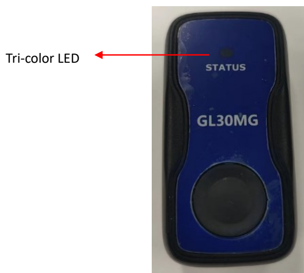
Figure 3. MICRO tri-color LED
