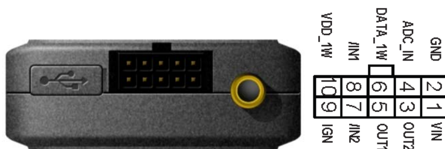
Figure . . The 10 PIN Connector on the GV65
