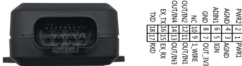
Figure 3. The 18-pin Connector on the GV620MG
