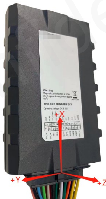
Figure 17. Motion Sensor Direction
