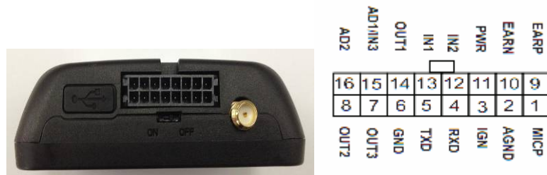
Figure 2. The 16 PIN Connector on the GV304N
