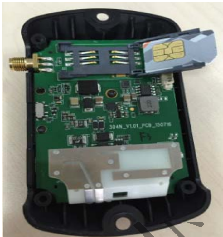
Figure 5. SIM Card Installation
