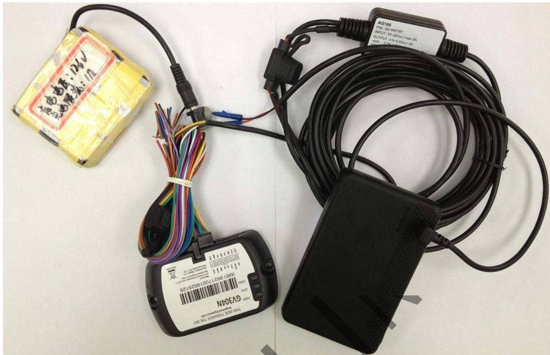
Figure 18. GV304N connection with Garmin GPS set
