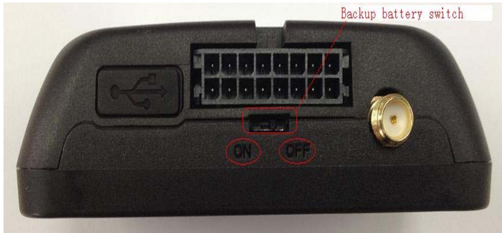
Figure 7. Switch and ON/OFF position
