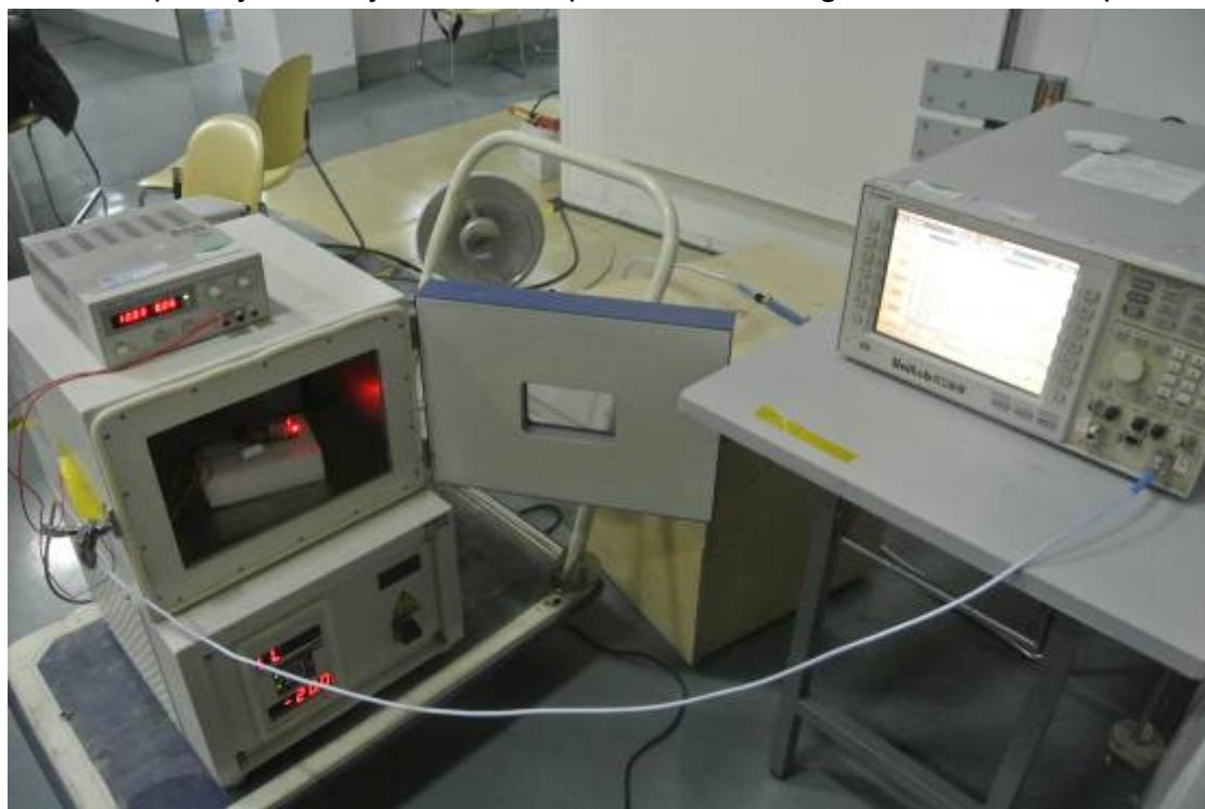
Radiated Spurious Measurement(below 30MHz) Setup
