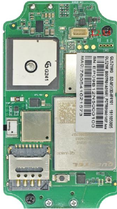
Figure 3. 4-pin Connector of the GL521MG
