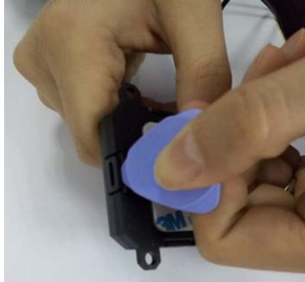
Figure 2. Opening the Case
