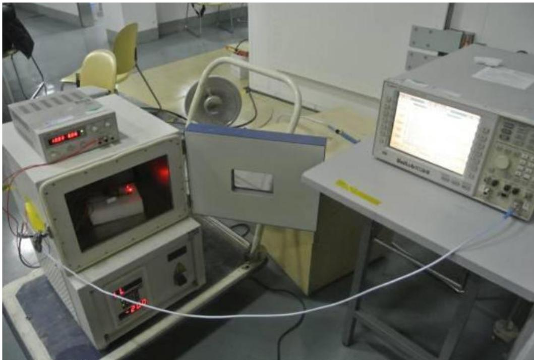
ERP Test, Radiated Spurious Measurement(Blow 30MHz) Setup
