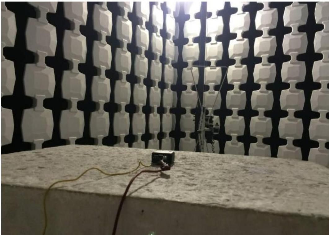
EIRP Test, Radiated Spurious Measurement (Above 1GHz) Setup
