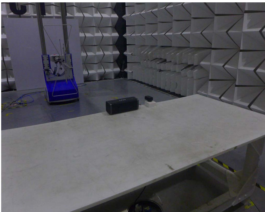
Radiated spurious emission Test Setup-2(Below 1GHz)
