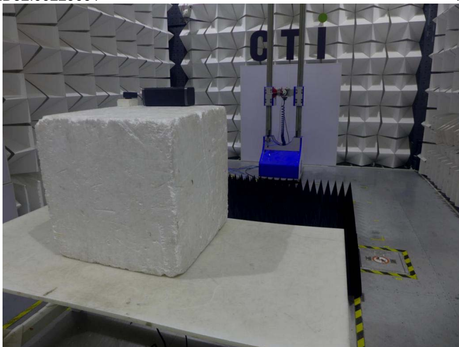
Radiated spurious emission Test Setup-3(Above 1GHz)
