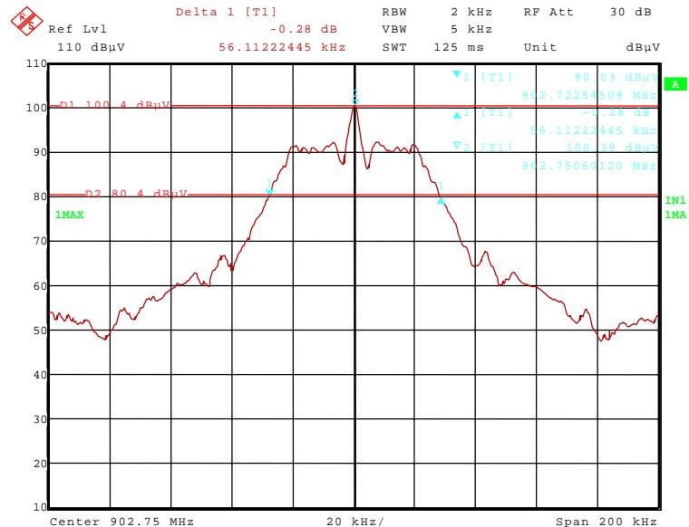
153142\_9.wmf: 20 dB bandwidth at the middle of the assigned frequency band:
