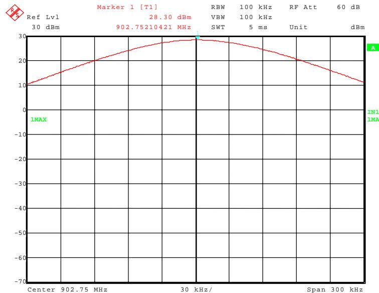
153142\_24.wmf: Maximum peak output power at the middle of the assigned frequency band:
