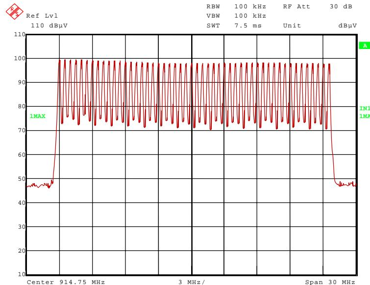
Remark: A smaller Resolution bandwidth was used in order to receive a better optical separation of the signal peaks.
