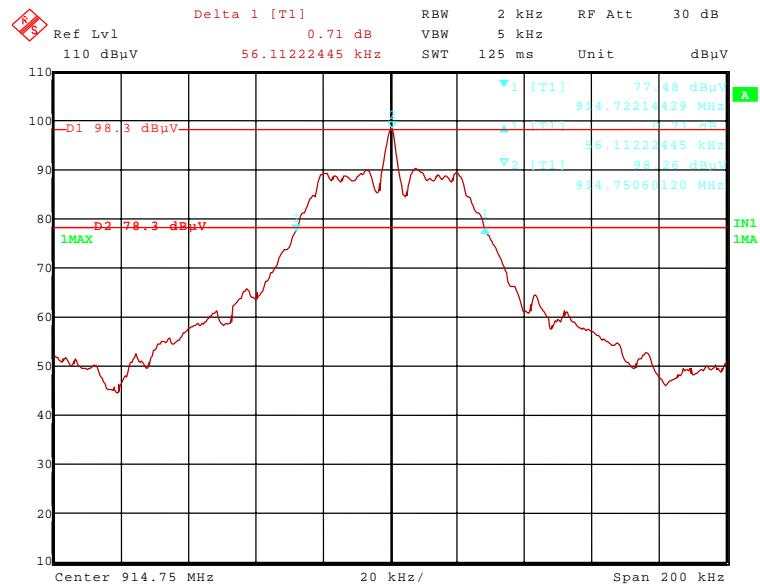
153142\_10.wmf: 20 dB bandwidth at the upper end of the assigned frequency band:
