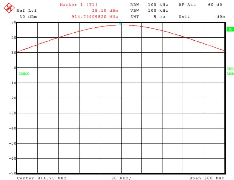
153142\_23.wmf: Maximum peak output power at the upper end of the assigned frequency band:
