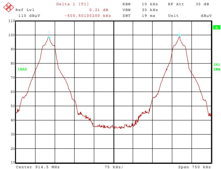
153142\_11.wmf: Channel separation at the upper end of the assigned frequency band:
