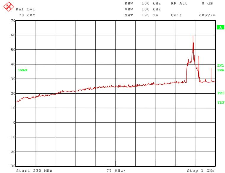
The following frequencies were found outside the restricted bands during the preliminary radiated emission test:
