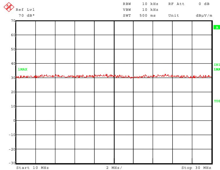
No significant frequencies above the noise floor of the system (max. 33 dB $\mu$ V/m (measured with peak detector) at 3 m distance) were found during the preliminary radiated emission test, so no measurements were carried out on the outdoor test site.
