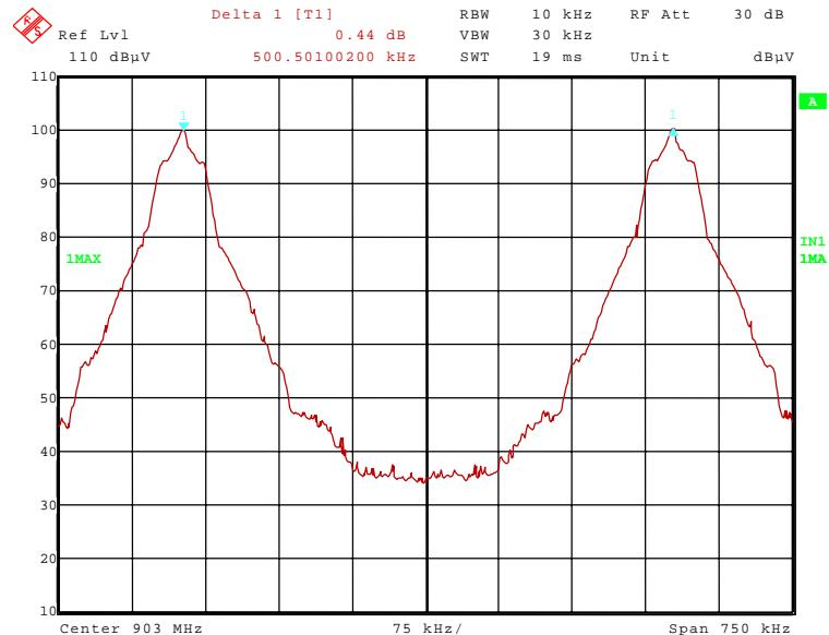
153142\_12.wmf: Channel separation at the middle of the assigned frequency band:
