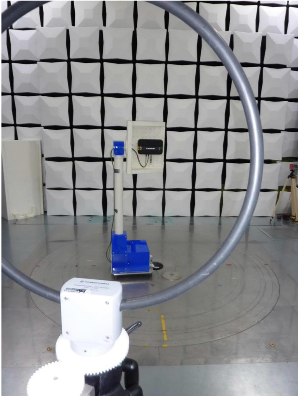
TN-UHF-Q180L300-NA-CDS, test setup semi anechoic chamber TX spurious emissions from 150 kHz to 30 MHz
