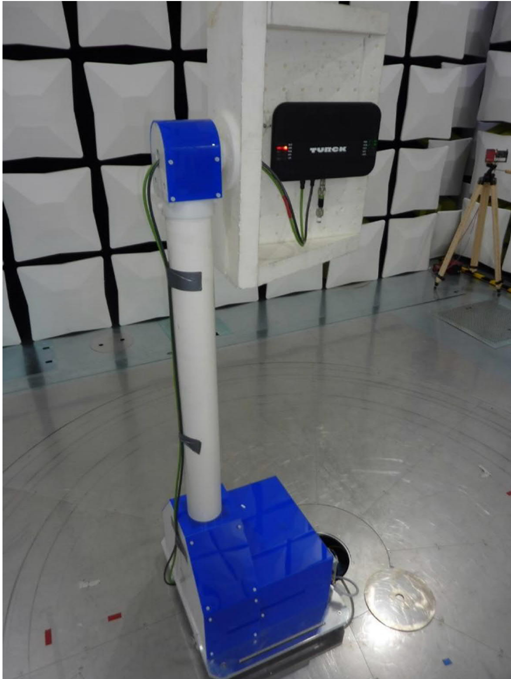
TN-UHF-Q180L300-NA-CDS, test setup semi anechoic chamber
