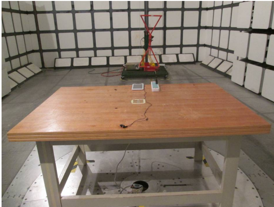
Radiated Emissions – Front View (30-1000 MHz)
