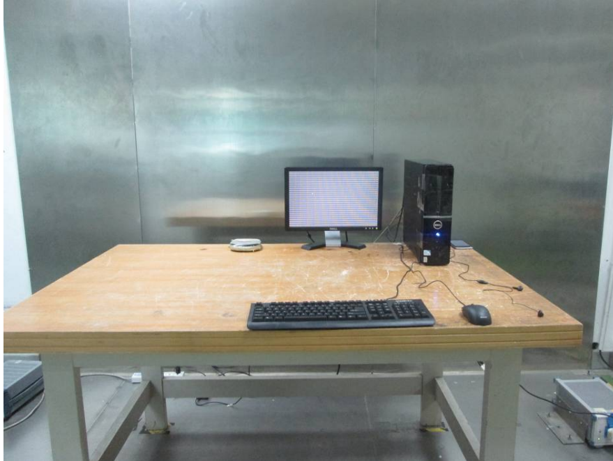
Conducted Emissions - Front View
