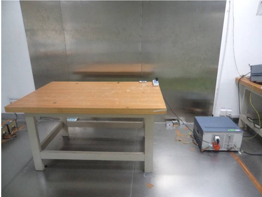
Conducted Emissions - Side View (Charging mode)
