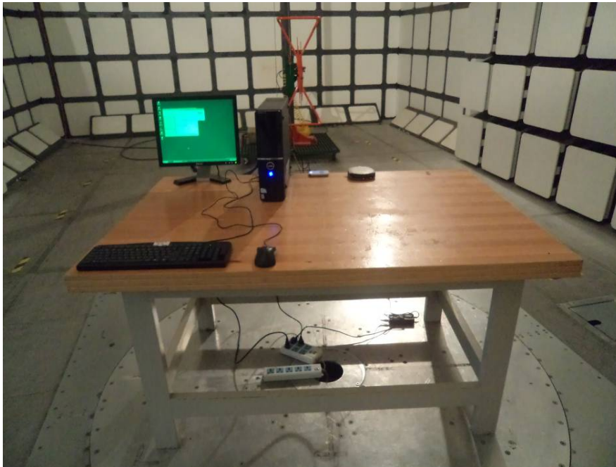
Radiated Emissions-Front View (downloading mode, 30-1000 MHz)
