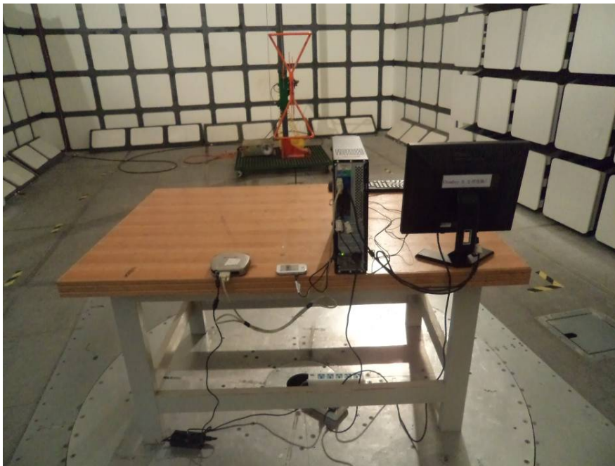
Radiated Emissions – Rear View (downloading mode, 30-1000 MHz)
