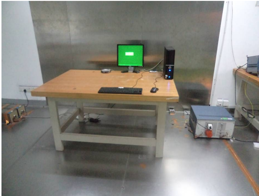
Conducted Emissions - Front View (downloading mode)
