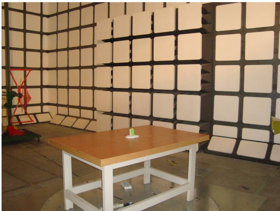
Below 1 GHz: Radiated Emissions - Rear View
