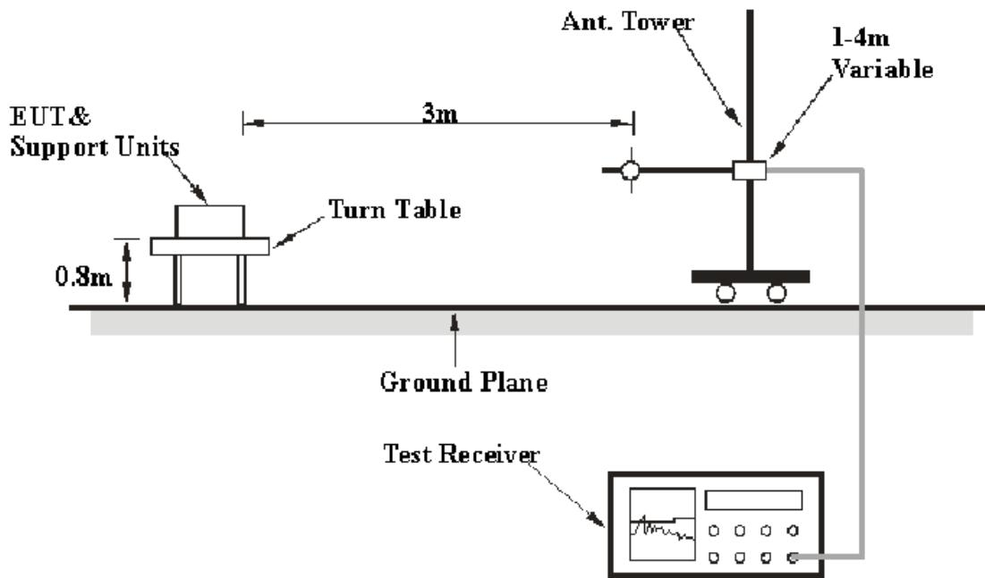
The radiated emission tests were performed in the 3 meters test site, using the setup accordance with the ANSI C63.4-2009. The specification used was the FCC Part 15.109 Class B limits.
