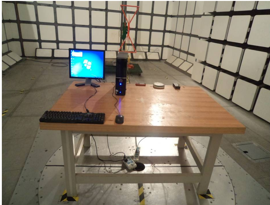
Radiated Emissions-Front View (downloading mode, 30-1000 MHz)
