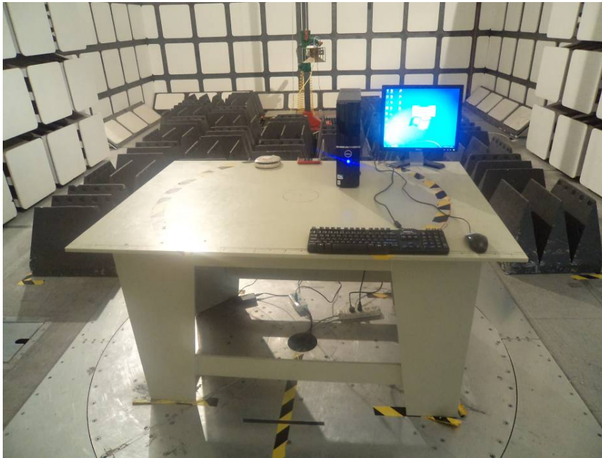
Radiated Emissions-Front View (downloading mode, 1-5GHz)
