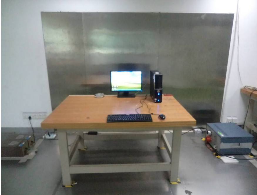
Conducted Emissions - Front View (downloading mode)
