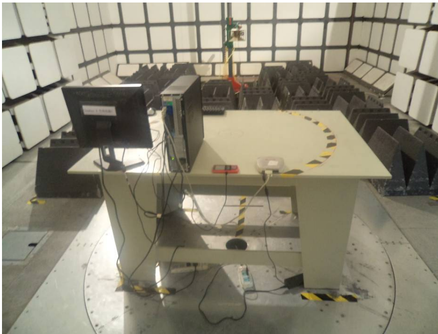
Radiated Emissions – Rear View (downloading mode, 1-5GHz)
