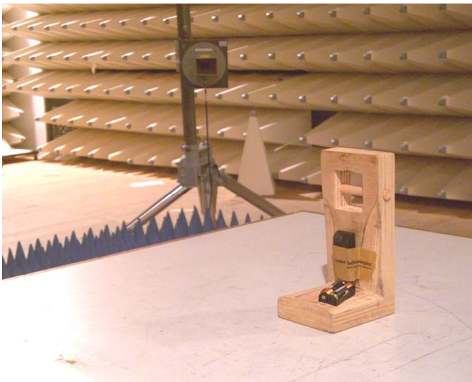
Fig. 5.2.4: Basic set-up for radiated emission test above 18 GHz @3m
