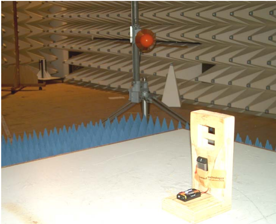
Fig. 5.2.3: Basic set-up for radiated emission 1 GHz – 18 GHz @ 3m
