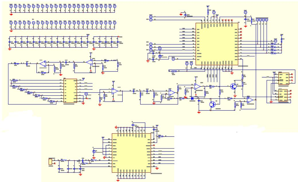
As shown in the schematic of our products, the signal of the interactive pen is collected by MUC, through a certain method of calculation, the coordinates of the tip position (X, Y) is fixed. There is a RF dongle on PC's USB put port, MCU control RF send out the cy6936 chip, RF dongle received from the board over the schematic board original signal, the USB transfer to PC.
