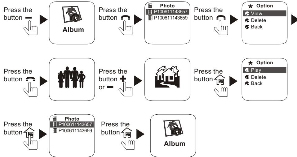
If you need to delete this picture, please select [Delete] and press the button , then select [Yes] and press the button to confirm. To return to the previous menu, you can also select [Back] and press the button .
