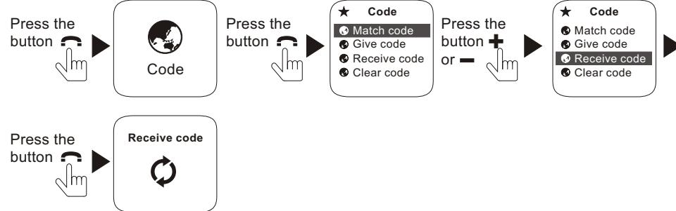
If the highlighted **success** appeared on the screen, it means that receive code is successful both of two indoor monitors. If the highlighted **failed** appeared, that means that it is to fail to receive code, please retry the step as above.
