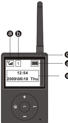
Please note that the system will go into the dark screen savers in 10s of time span without any button is pressed until you press the button to relight the screen again , meanwhile the power LED is slowly flashing red.
