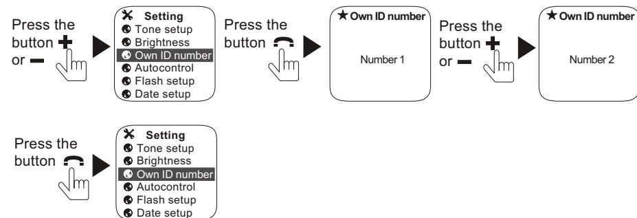
This system allows up to 3 video indoor monitors to connect with 1 outdoor camera, therefore each indoor monitor needs to program the different ID number respectively, otherwise the same ID number maybe result in some unknown malfunctions.
