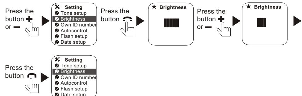
It is useless to press the button if the brightness of TFT display reaches to Min. Value or Max. Value.
