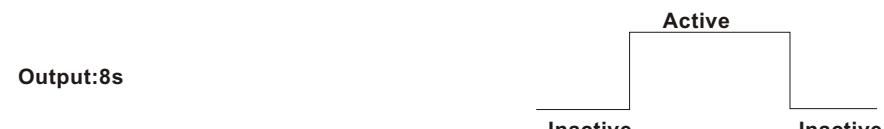
The dry contact is kept under active or inactive condition if the unlock button is pressed on indoor monitor, with active duration is 8s.
