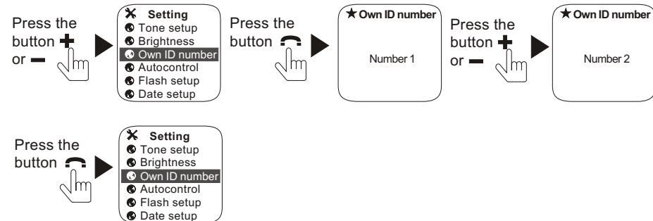
This system allows up to 3 video indoor monitors to connect with 1 outdoor camera, therefore each indoor monitor needs to program the different ID number respectively, otherwise the same ID number maybe result in some unknown malfunctions.
