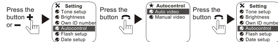
If the **Auto video record** mode is selected, when the call button is pressed on the outdoor camera, and then your indoor unit will sound melodies meanwhile the visitor's image will display on the screen, in the upper left of the screen, an superimposed icon indicates that a real time video record is underway.
