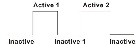
The dry contact is kept under active or inactive condition if the unlock button is pressed on indoor monitor, with Active 1 duration is 600ms, Inactive 1 duration is 400ms and Active 2 duration is 800ms.
