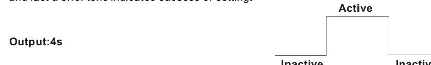
The dry contact is kept under active or inactive condition if the unlock button is pressed on indoor monitor, with active duration is 4s.
