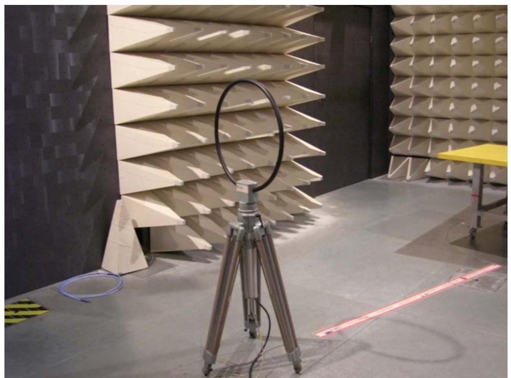
For radiated emissions 30MHz~1GHz
