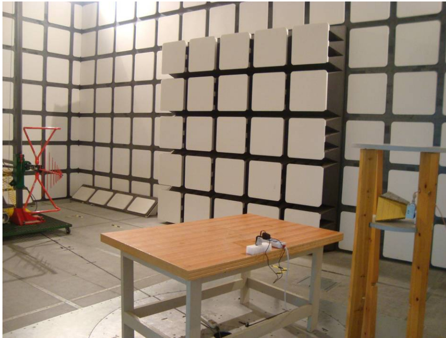
Below 1 GHz: Radiated Emissions –Rear View
