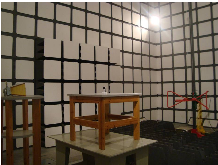
Below 1GHz: Spurious Radiated Emissions - Rear View
