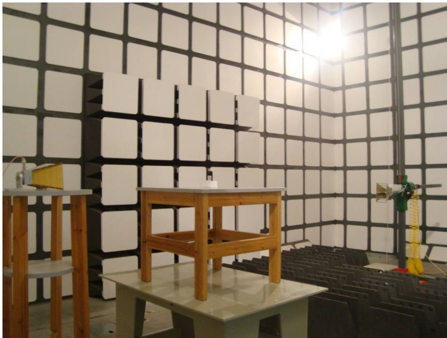
Above 1GHz: Spurious Radiated Emissions - Rear View
