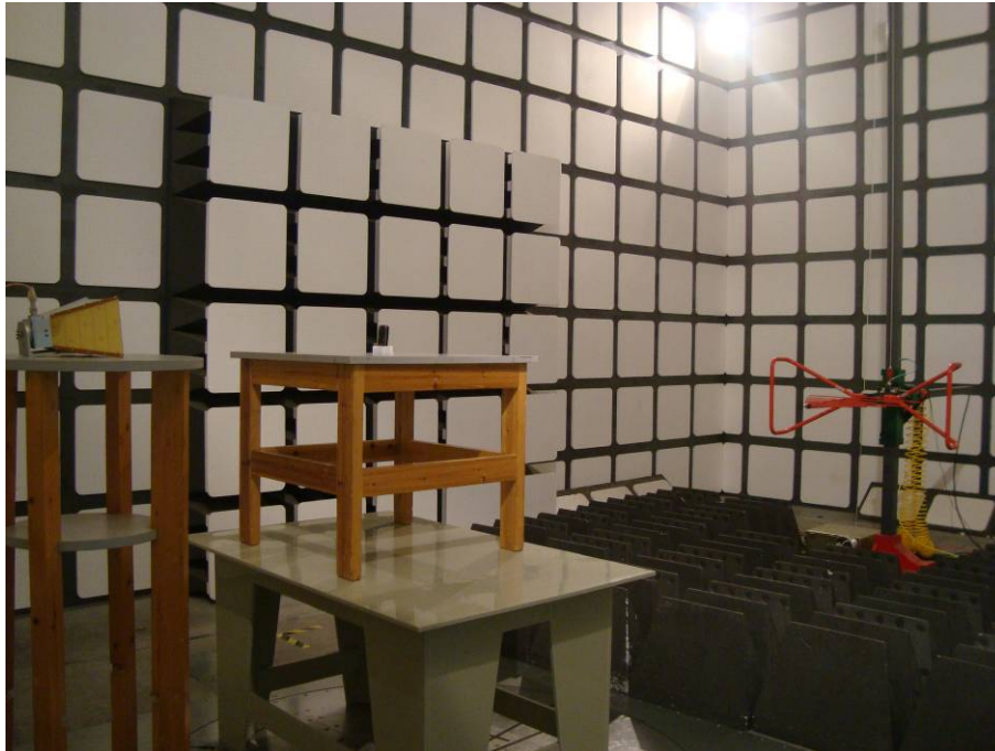
Below 1GHz: Spurious Radiated Emissions - Front View
