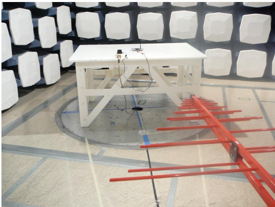
**Radiated Emission below 1 GHz Rear View (Dipole Antenna)**
