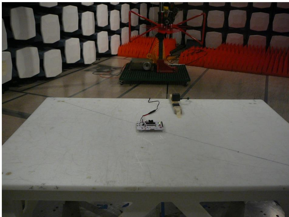
**Radiated Emission above 1 GHz Front View (Integrated ceramic chip Antenna)**
