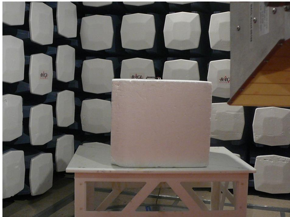
**Radiated Emission above 1 GHz Rear View (Integrated ceramic chip Antenna)**
