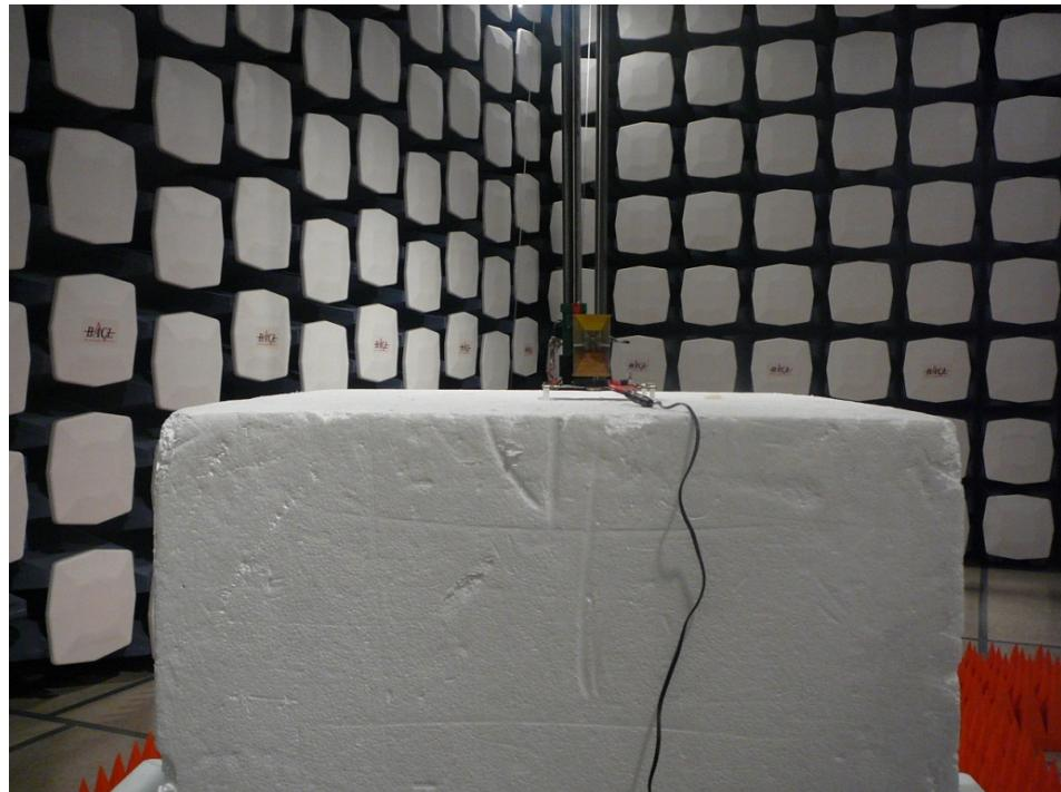
**Radiated Emission below 1 GHz Front View (Dipole Antenna)**
