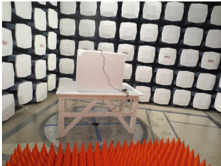
**Radiated Emission above 1 GHz Rear View (PCB Antenna)**
