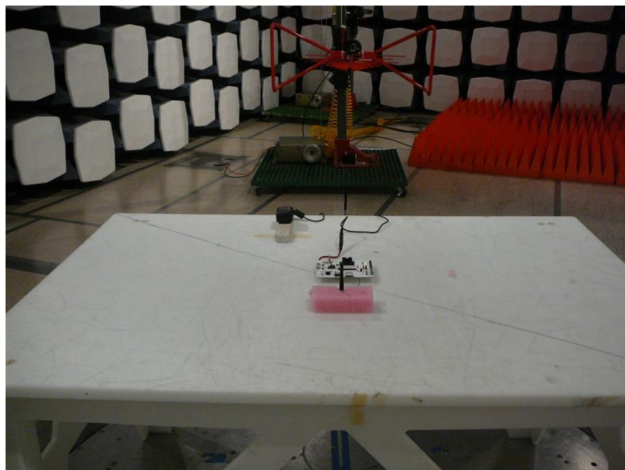
**Radiated Emission above 1 GHz Front View (Dipole Antenna)**
