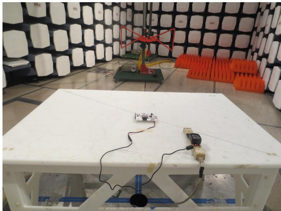
**Radiated Emission above 1 GHz Front View (PCB Antenna)**
