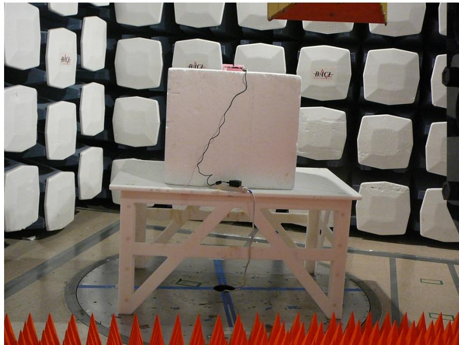
**Radiated Emission above 1 GHz Rear View (Dipole Antenna)**
