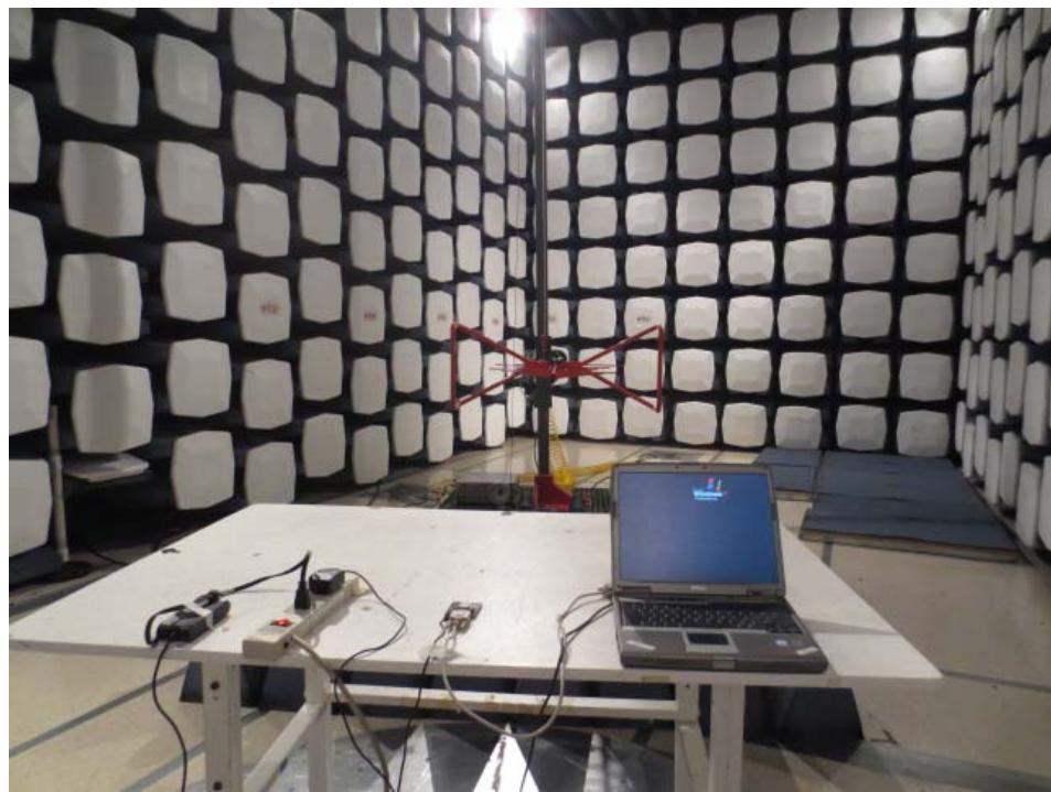
**15.5 Radiated Emission above 1 GHz Rear View at 3 Meter**
