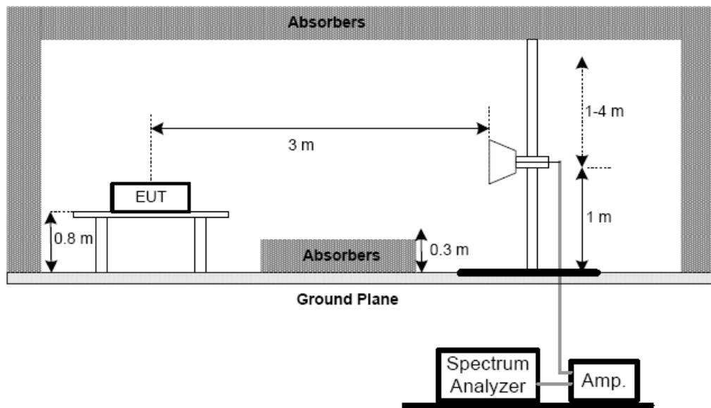
(C) For radiated emissions below 30MHz
