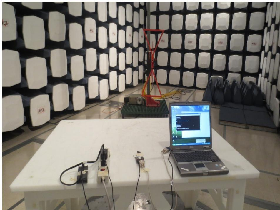
**15.8 Radiated Emission above 1 GHz Rear View at 3 Meter – EUT with PCB Antenna**
