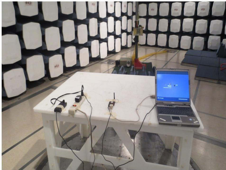
**15.6 Radiated Emission Front View at 3 Meter – EUT with PCB Antenna**
