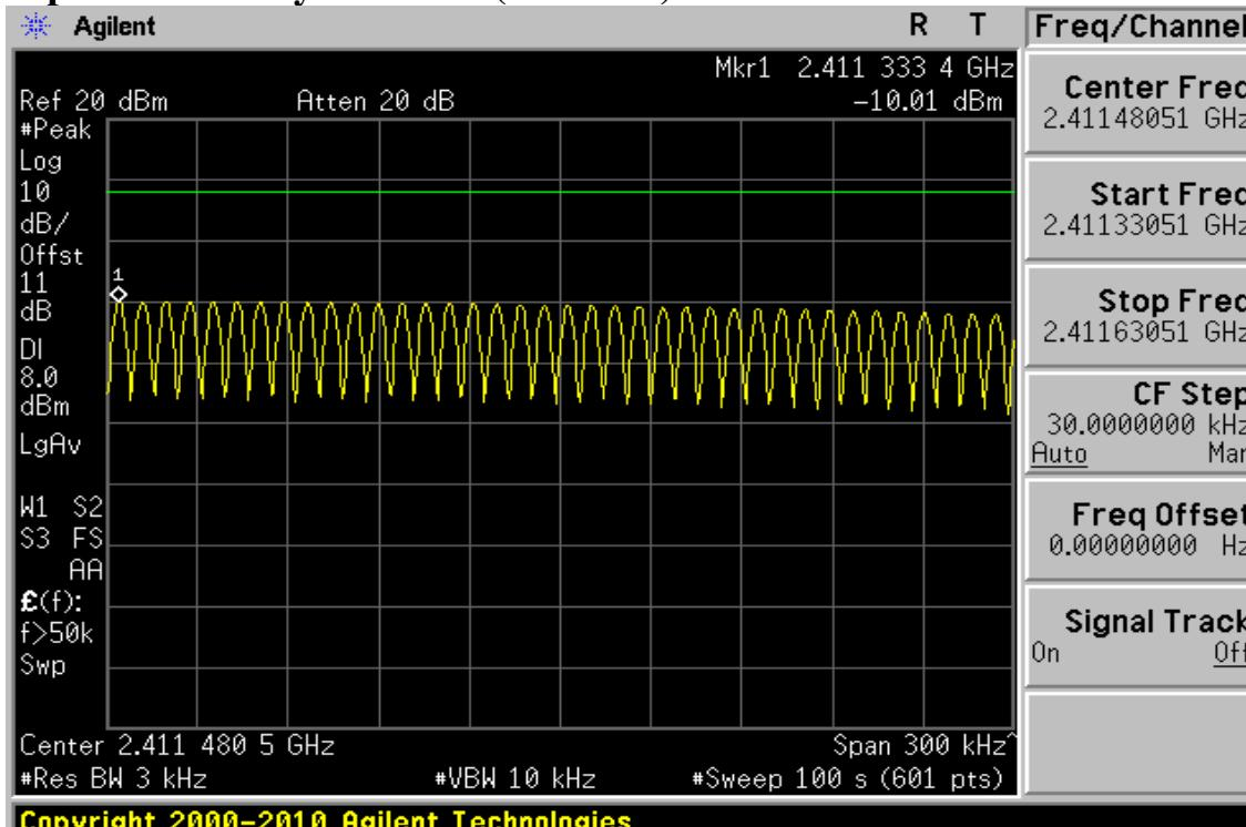
**Power Spectral Density Test Plot (CH-Mid)**
