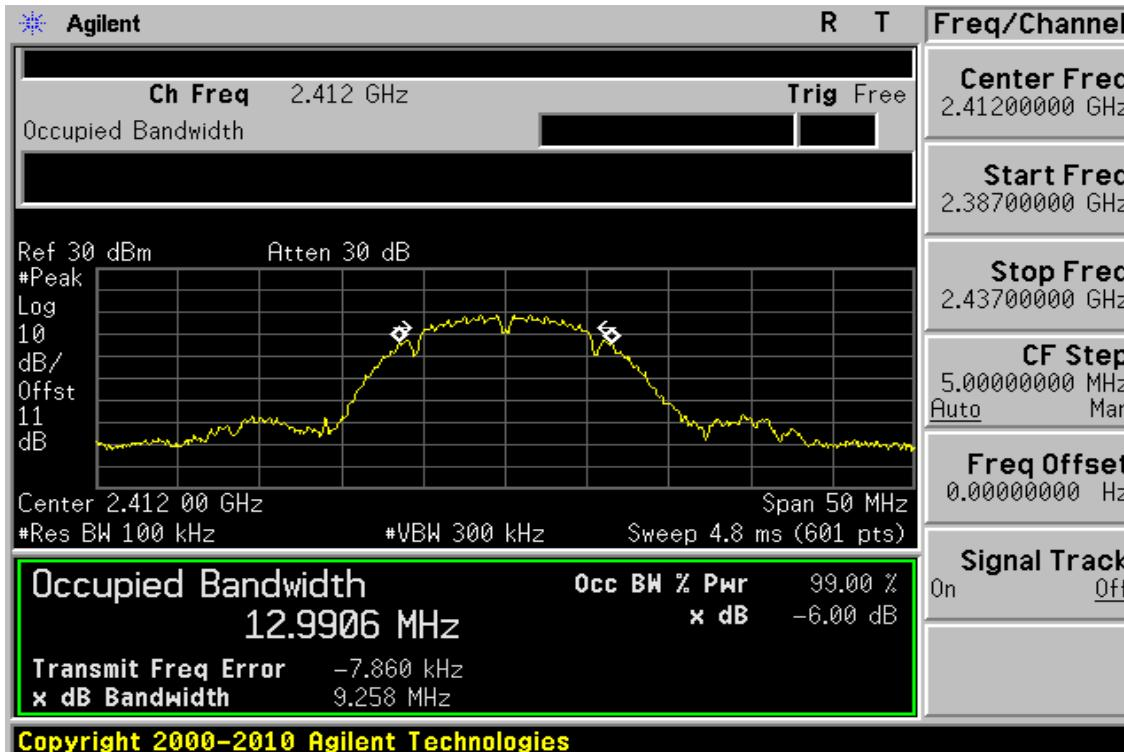
**6dB Bandwidth Test Data CH-Mid**
