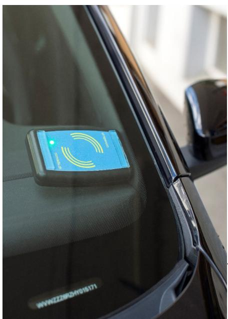
Please make sure, that the unit is fixed securely to not become loose, even during a crash. Please clean the mounting place with alcohol before taping it onto the glass. I The device is including a high frequency cell phone antenna and other RF antennas and therefore it must be placed at least 20 cm away from the passenger body in its usual position. Please also locate it 20 cm away from sensitive electronic parts and wires of the vehicle and from any other RF antenna.
