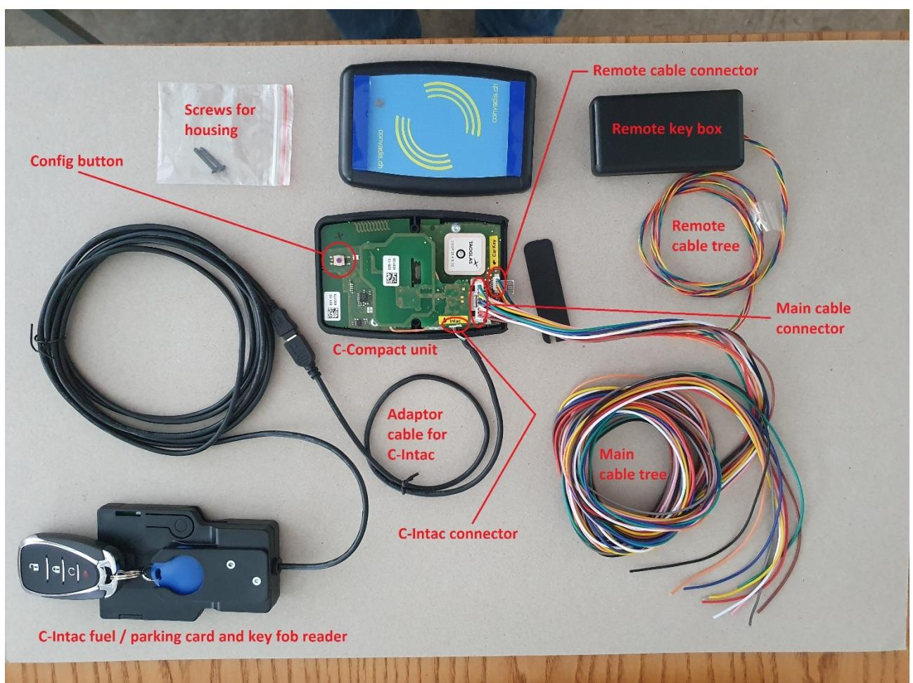
The unit includes a 10 pin connector with multiple hw configurable signal routing options and an additional connector for connecting remote keys of the car (for lock/ unlock and for immobilizer function on cars with keyless start system).
