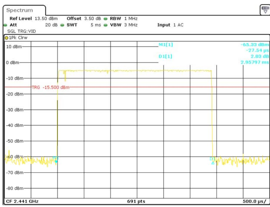
**Pulse time, High Channel, DH5**
