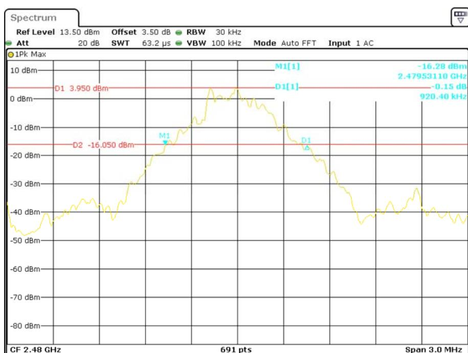
**EDR ( $\pi/4$ -DQPSK): Low Channel**
