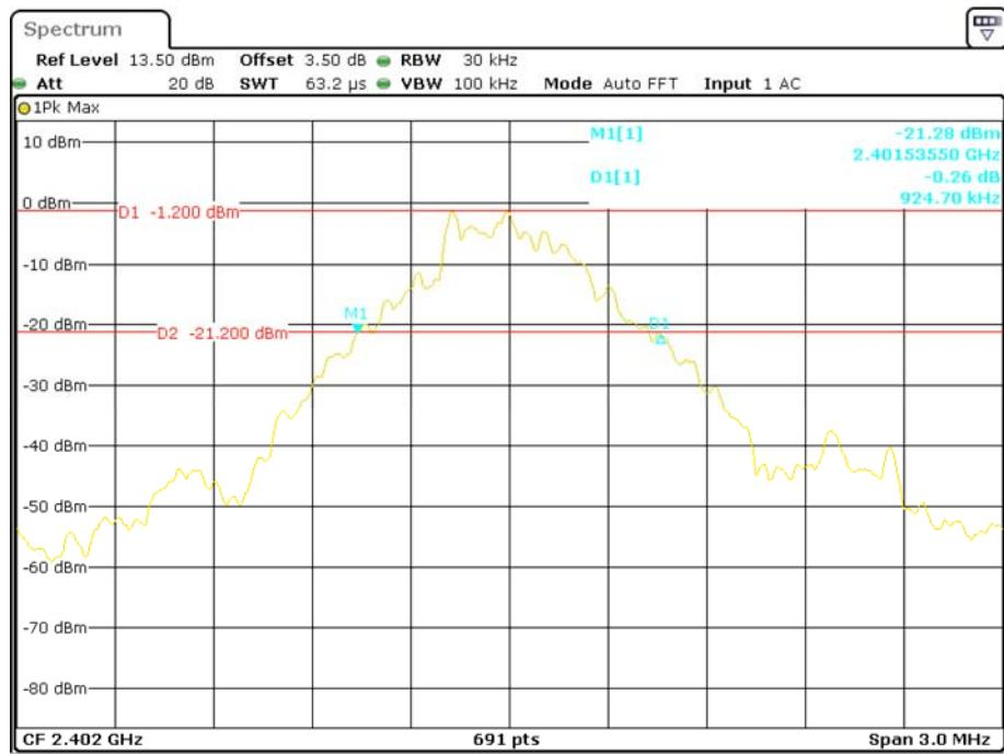
**BDR (GFSK): Middle Channel**
