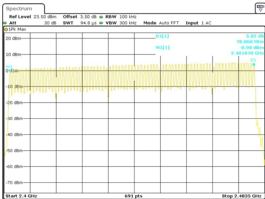
**EDR ( $\pi/4$ -DQPSK): Number of Hopping Channels**
