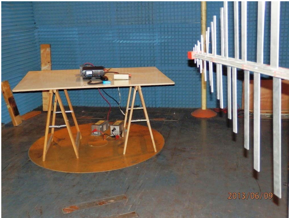
Test Setup for Field Strength of Spurious Emission/ 1
