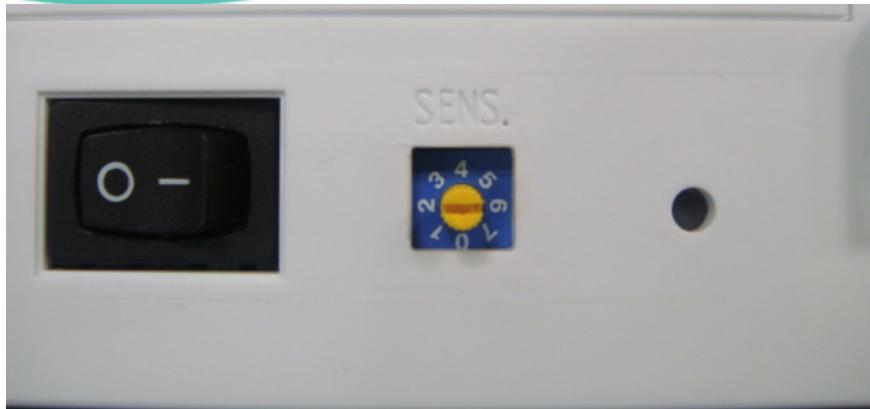
**Make sure the switch is clicked in place. If it is in between settings the sensor will behave unpredictably.**
