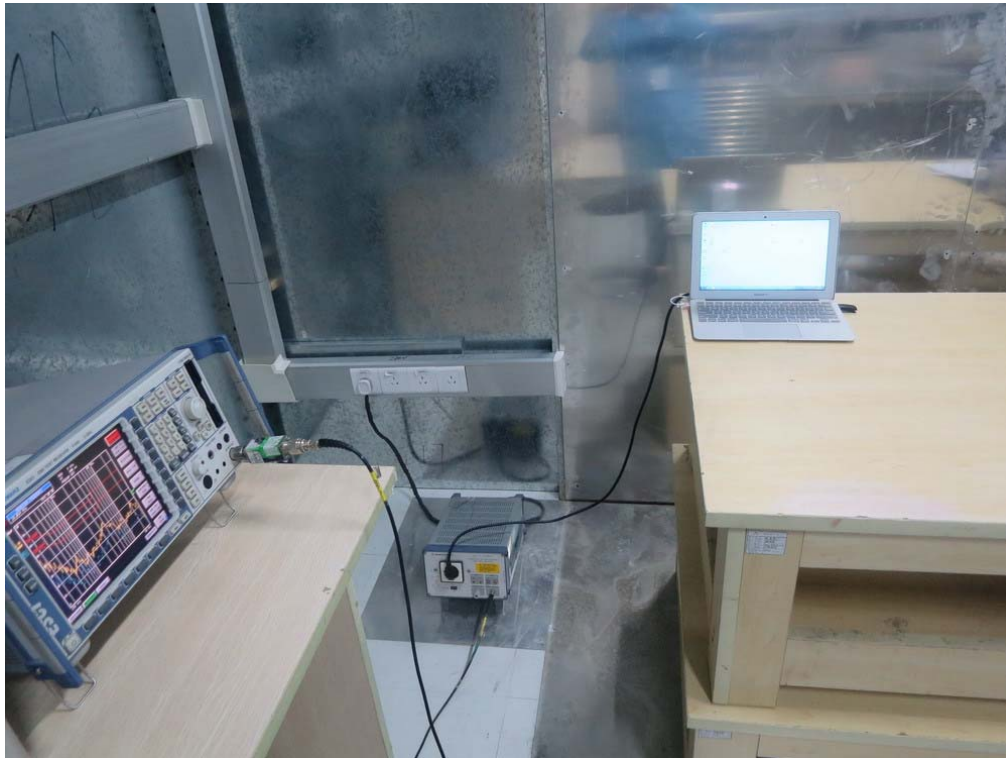
FCC RADIATED EMISSION TEST SETUP
