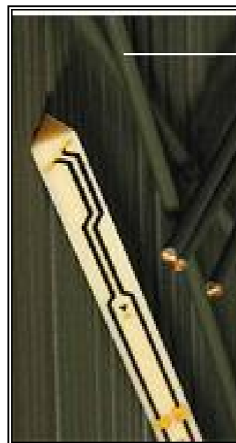
Inside View of SN11/09 EP100 E-field Probe
