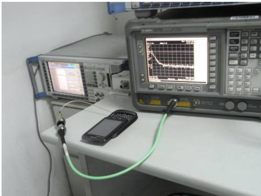
CONDUCTED SPURIOUS EMISSION TEST SETUP
