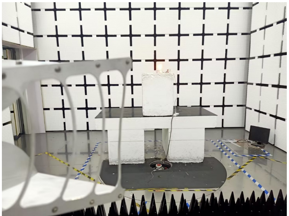
Radiation Emission Test Setup (1GHz to 18GHz)
