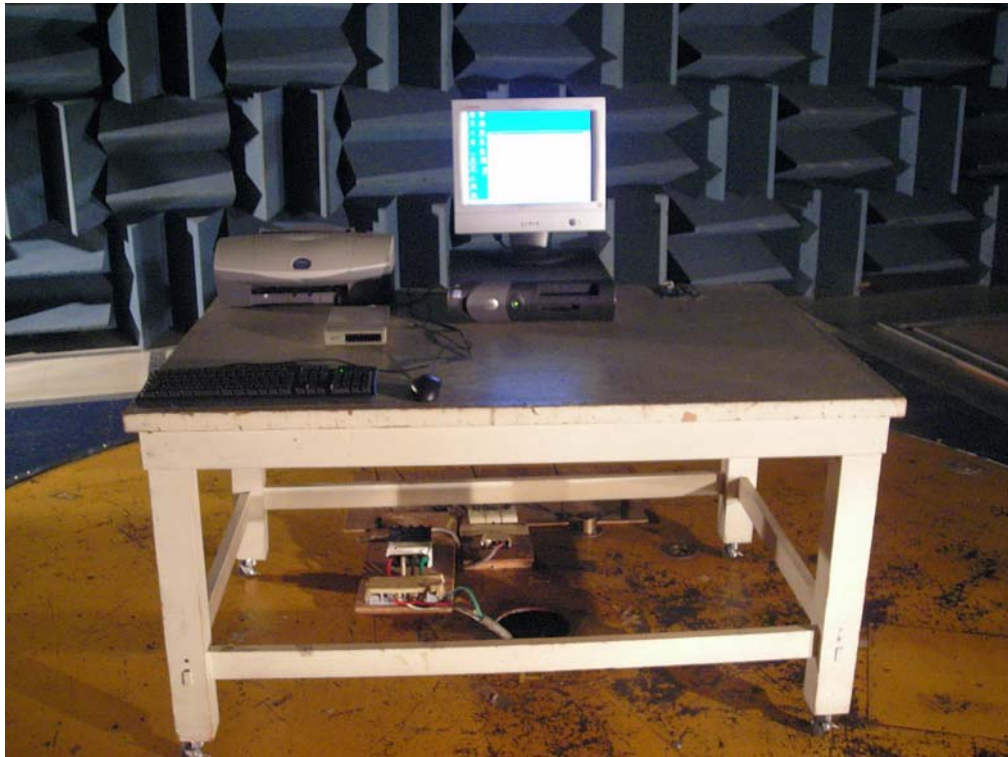
Photo 1.2 Setup with Maximized RFI Field Strength Measurement <30MHz to 1000MHz>
