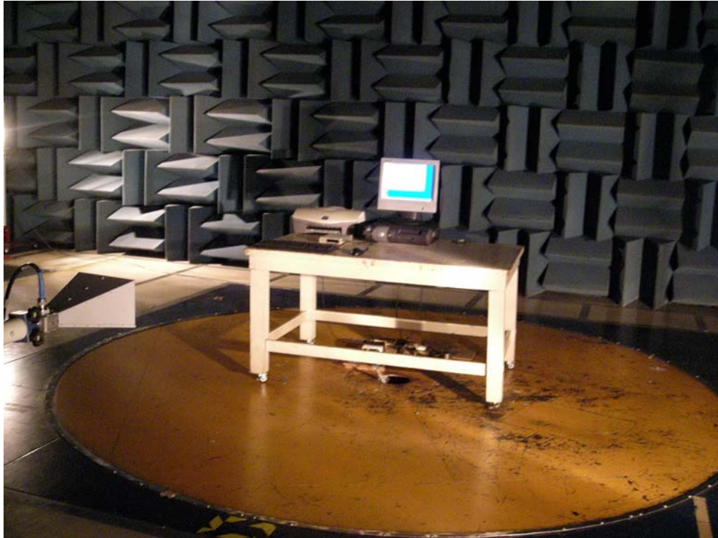
Photo 1.3 Setup with Maximized RFI Field Strength Measurement <1000MHz to 26500MHz>
