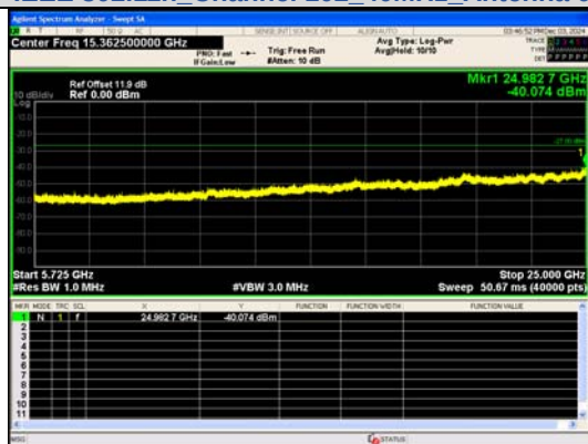
Spurious Emission:5725~25000.0 MHz IEEE 802.11n_Channel 102_40MHz_Antenna 0
