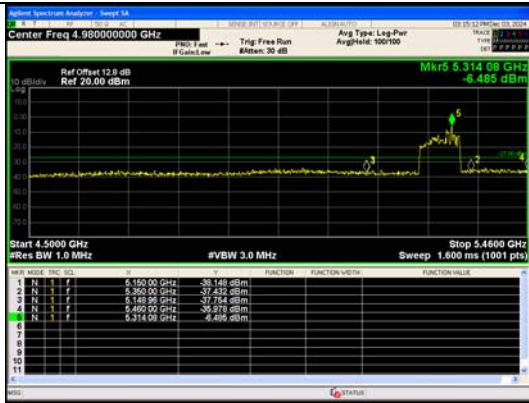
Out Of Band Emission IEEE 802.11ac Channel 58 80MHz Antenna 0
