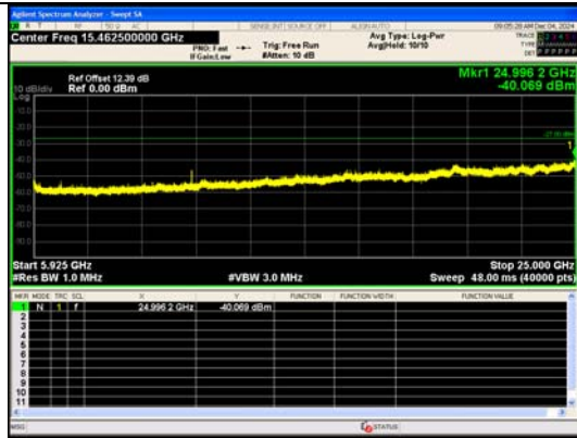
Spurious Emission:5925~25000.0 MHz IEEE 802.11ac Channel 149 20MHz Antenna 0
