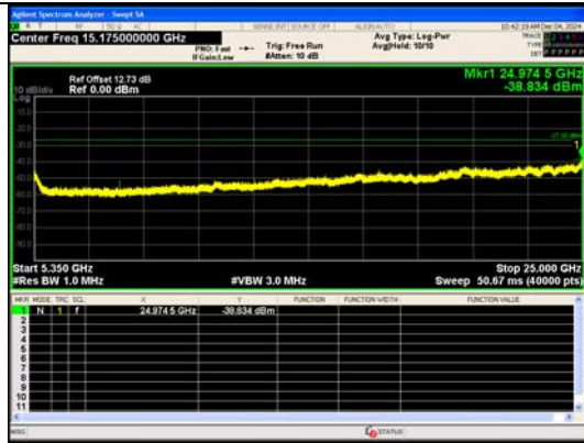
Spurious Emission:5350~25000.0 MHz IEEE 802.11n Channel 52 20MHz Antenna 0
