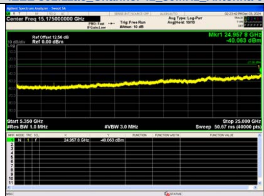
Spurious Emission:5350~25000.0 MHz IEEE 802.11ac_Channel 42_80MHz_Antenna 0
