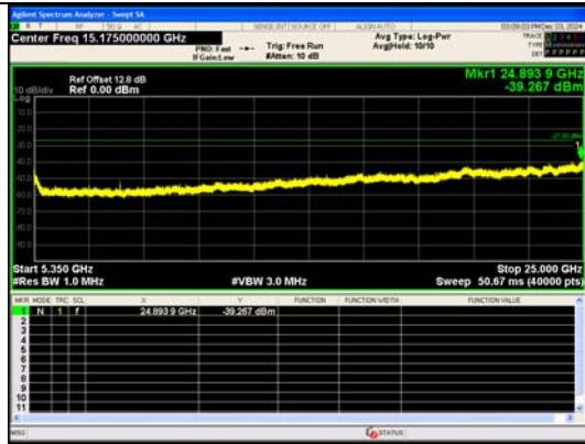
Spurious Emission:5350~25000.0 MHz IEEE 802.11ac Channel 54 40MHz Antenna 0
