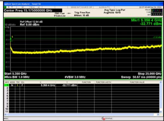
Spurious Emission:5350~25000.0 MHz IEEE 802.11a_Channel 64_20MHz_Antenna 0
