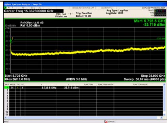
Spurious Emission:5725~25000.0 MHz IEEE 802.11ac_Channel 140_20MHz_Antenna 0
