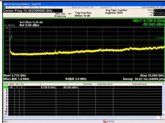
Spurious Emission:5725~25000.0 MHz IEEE 802.11a Channel 140 20MHz Antenna 0
