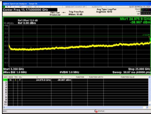
Spurious Emission:5350~25000.0 MHz IEEE 802.11n_Channel 54_40MHz_Antenna 0
