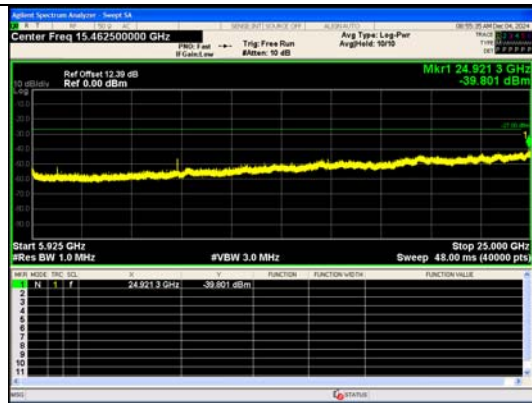
Spurious Emission:5925~25000.0 MHz IEEE 802.11a_Channel 149_20MHz_Antenna 0
