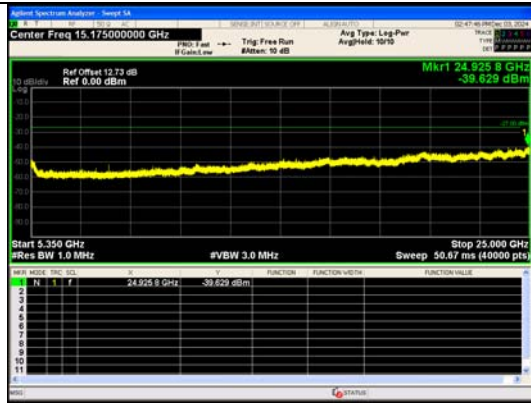
Spurious Emission:5350~25000.0 MHz IEEE 802.11ac_Channel 52_20MHz_Antenna 0
