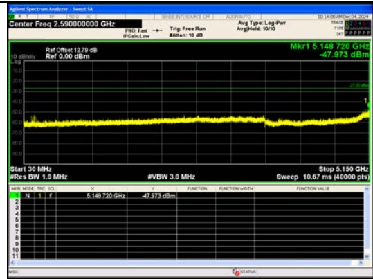
Spurious Emission:30.0~5150 MHz IEEE 802.11n Channel 38 40MHz Antenna 0
