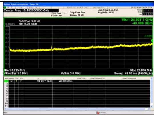
Spurious Emission:5925~25000.0 MHz IEEE 802.11ac_Channel 151_40MHz_Antenna 0
