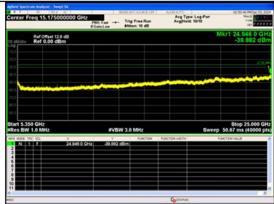
Spurious Emission:5350~25000.0 MHz IEEE 802.11ac_Channel 56_20MHz_Antenna 0
