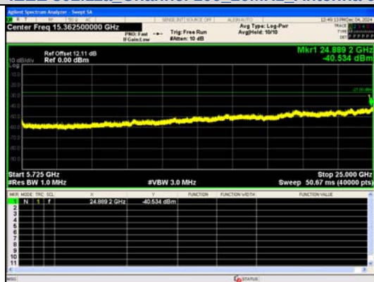
Spurious Emission:5725~25000.0 MHz IEEE 802.11a_Channel 100_20MHz_Antenna 0
