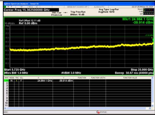
Spurious Emission:5725~25000.0 MHz IEEE 802.11ac_Channel 100_20MHz_Antenna 0
