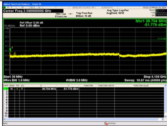
Spurious Emission:30.0~5150 MHz IEEE 802.11n_Channel 62_40MHz_Antenna 0
