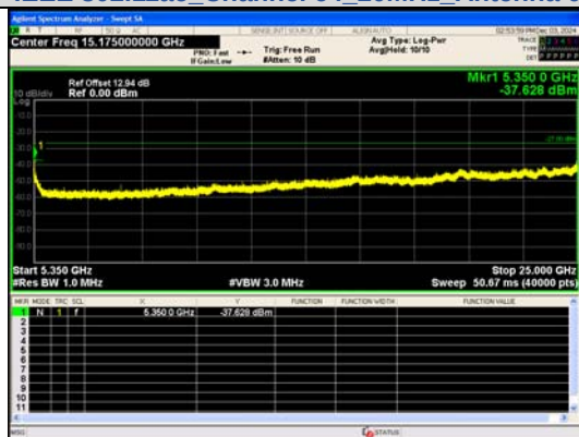
Spurious Emission:5350~25000.0 MHz IEEE 802.11ac_Channel 64_20MHz_Antenna 0
