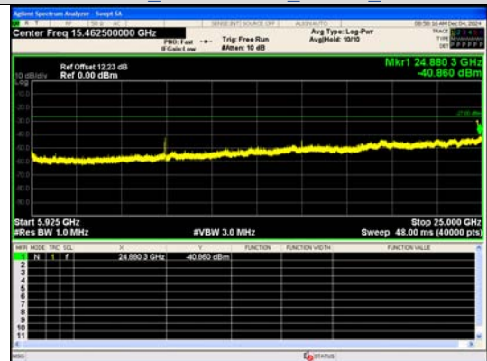
Spurious Emission:5925~25000.0 MHz IEEE 802.11a_Channel 157_20MHz_Antenna 0
