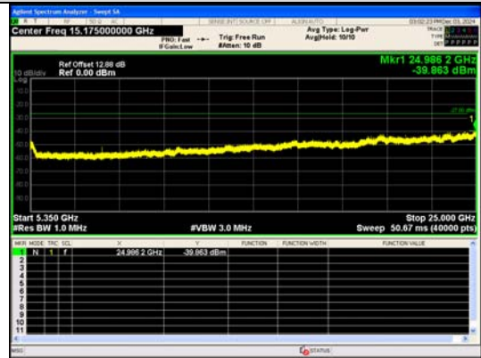
Spurious Emission:5350~25000.0 MHz IEEE 802.11n_Channel 62_40MHz_Antenna 0
