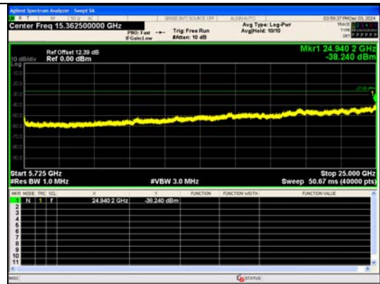
Spurious Emission:5725~25000.0 MHz IEEE 802.11ac_Channel 118_40MHz_Antenna 0
