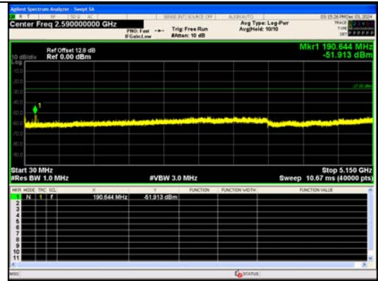
Spurious Emission:30.0~5150 MHz IEEE 802.11ac Channel 58 80MHz Antenna 0
