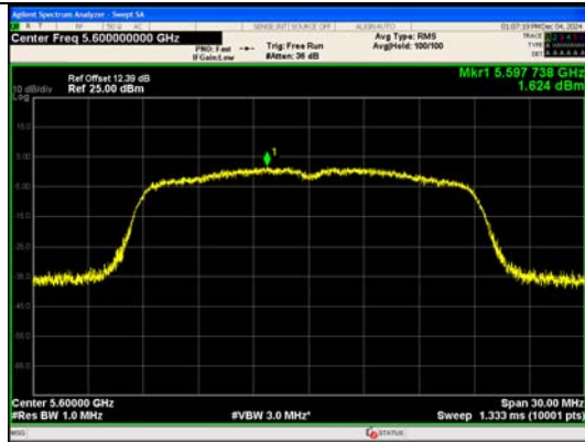
IEEE 802.11ac Channel 120 20MHz Antenna 0
