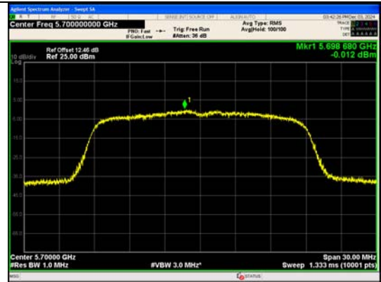
IEEE 802.11ac Channel 140 20MHz Antenna 0
