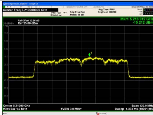
IEEE 802.11ac Channel 42 80MHz Antenna 0
