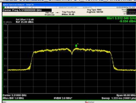
IEEE 802.11ac Channel 102 40MHz Antenna 0
