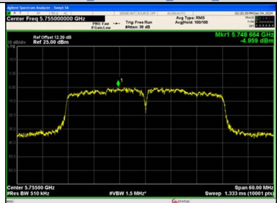
IEEE 802.11ac Channel 151 40MHz Antenna 0
