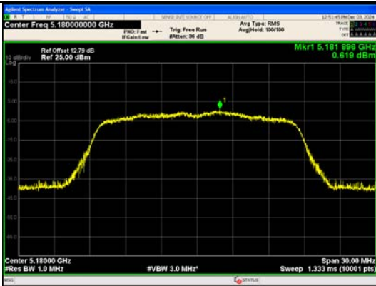
IEEE 802.11a Channel 36 20MHz Antenna 0
