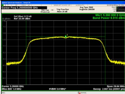
Conducted AVG output power IEEE 802.11n 20 Channel 52 Antenna 0
