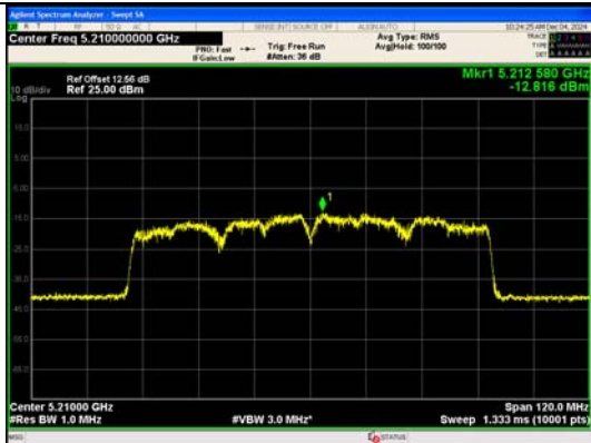
IEEE 802.11ac Channel 42 80MHz Antenna 0
