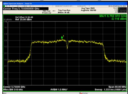
IEEE 802.11ac Channel 151 40MHz Antenna 0
