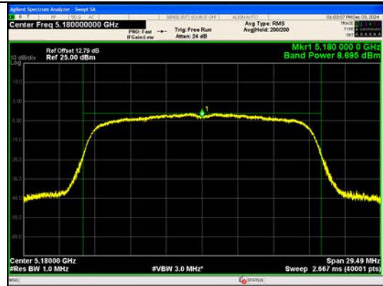
Conducted AVG output power IEEE 802.11n 20 Channel 36 Antenna 0
