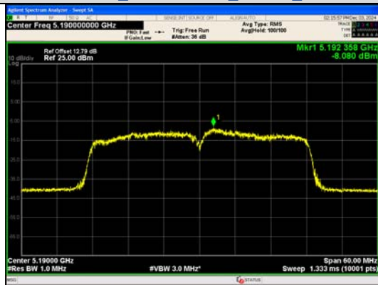
IEEE 802.11ac Channel 38 40MHz Antenna 0
