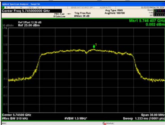
IEEE 802.11ac Channel 149 20MHz Antenna 0
