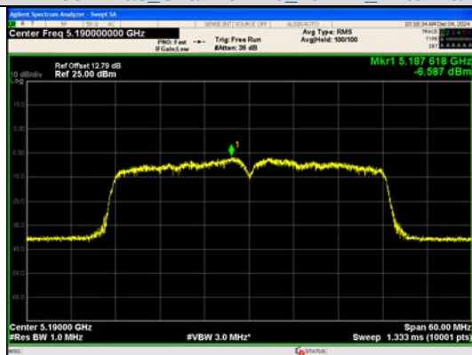
IEEE 802.11ac Channel 38 40MHz Antenna 0
