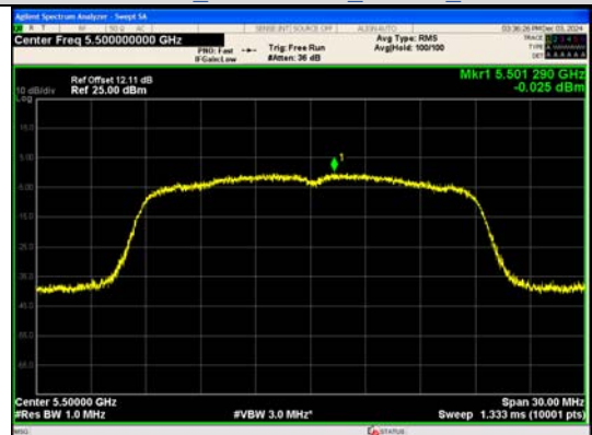
IEEE 802.11ac Channel 100 20MHz Antenna 0
