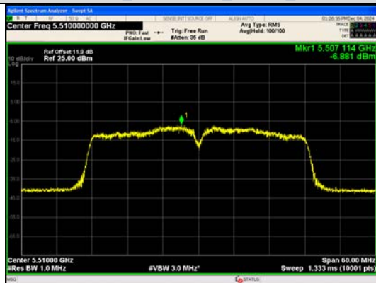
IEEE 802.11ac Channel 102 40MHz Antenna 0
