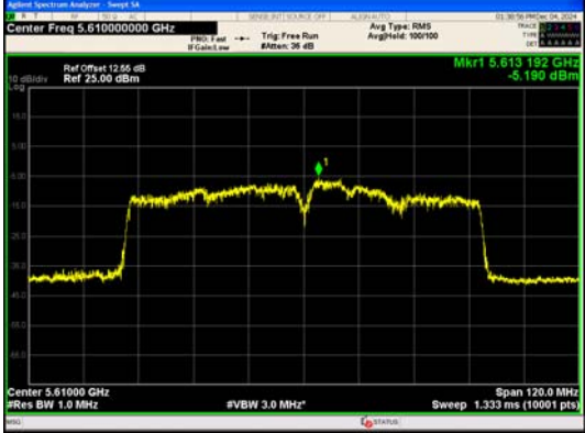
IEEE 802.11ac Channel 122 80MHz Antenna 0
