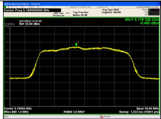
IEEE 802.11ac Channel 36 20MHz Antenna 0
