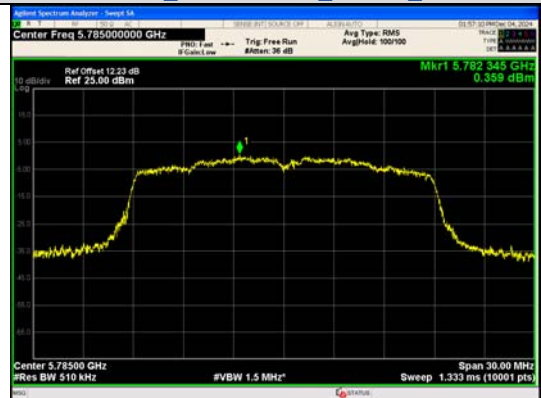
IEEE 802.11ac Channel 157 20MHz Antenna 0
