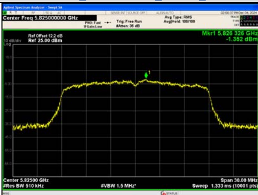
IEEE 802.11ac Channel 165 20MHz Antenna 0
