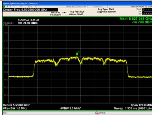
IEEE 802.11ac Channel 106 80MHz Antenna 0
