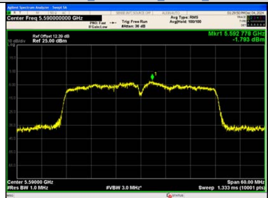
IEEE 802.11ac Channel 118 40MHz Antenna 0
