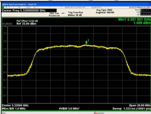
IEEE 802.11ac Channel 64 20MHz Antenna 0
