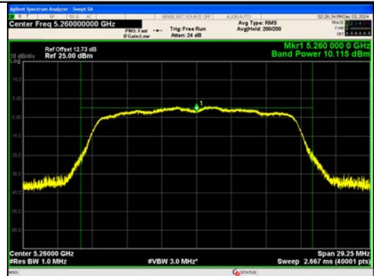
Conducted AVG output power IEEE 802.11a Channel 52 Antenna 0
