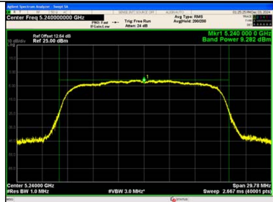
Conducted AVG output power IEEE 802.11n 20 Channel 48 Antenna 0
