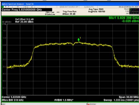
IEEE 802.11ac Channel 165 20MHz Antenna 0
