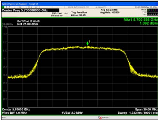
IEEE 802.11a Channel 140 20MHz Antenna 0
