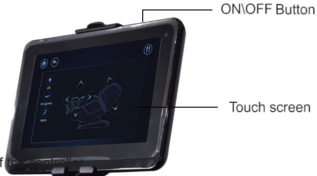
1. Power switch on the top of the controller
