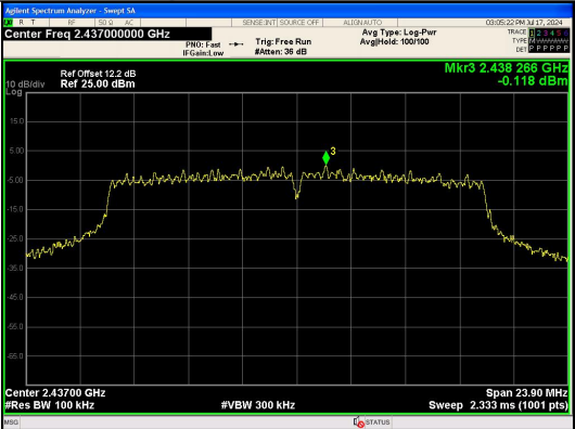
In-Band Reference Level IEEE 802.11g_Channel 6_20MHz_Antenna 0
