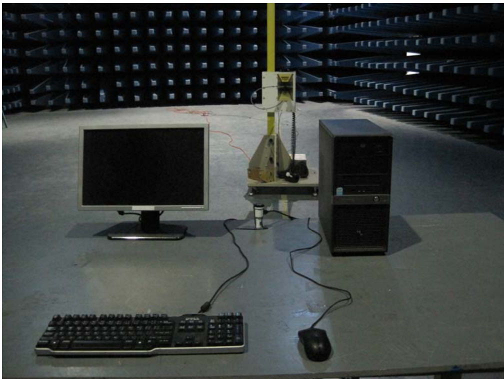
Radiated Spurious Emissions Test Setup (Above 1GHz)
