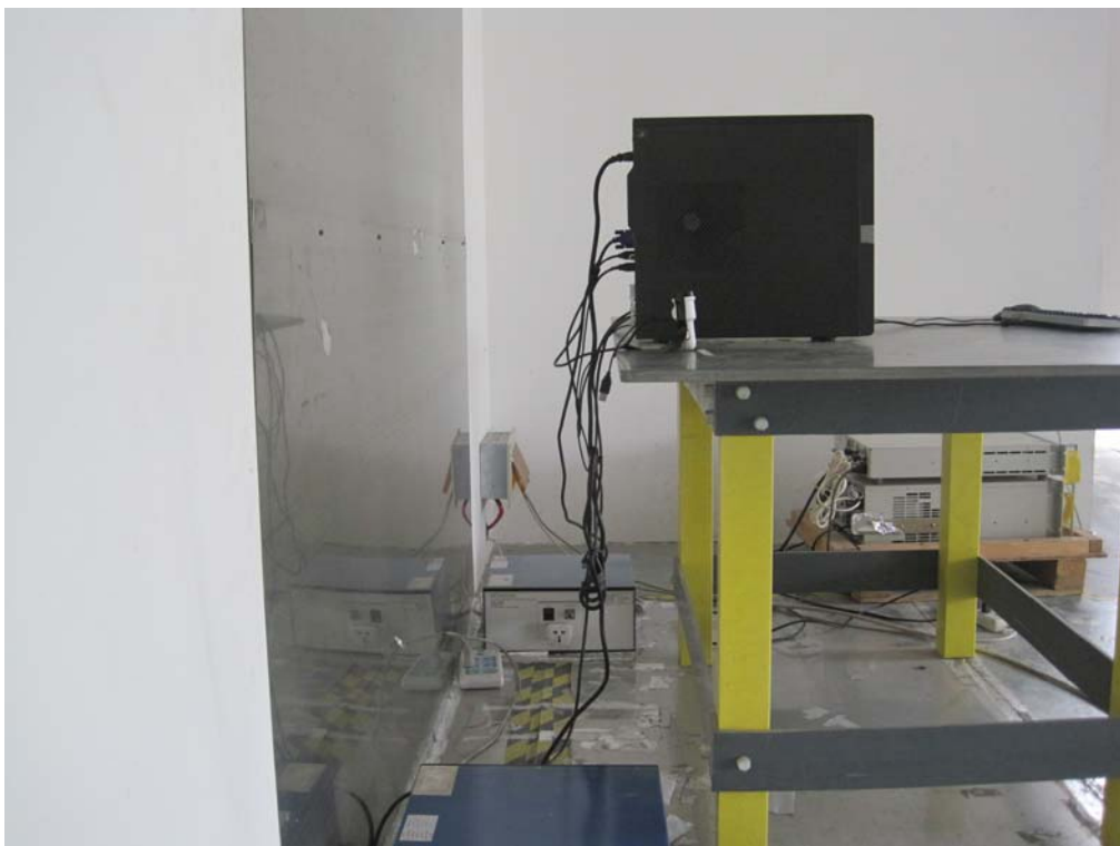
Conducted Emissions Test Setup Side View
