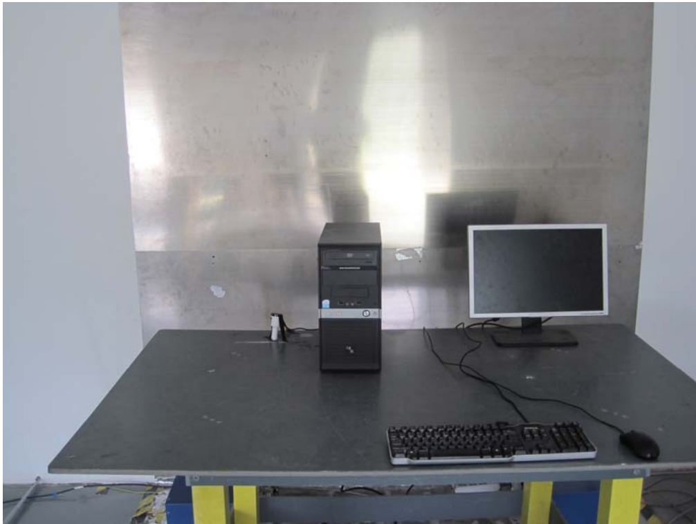
Conducted Emissions Test Setup Front View
