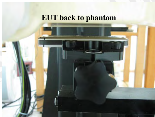
Fig.7 Body worn- EUT Back to flat phantom and distance between flat phantom and mobile phone is 1.5 cm
